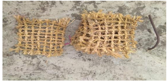
Figure 2 PSG specimens of 6 mm thickness and 12 mm x 12 mm aperture and 200 mm x 200 mm size
