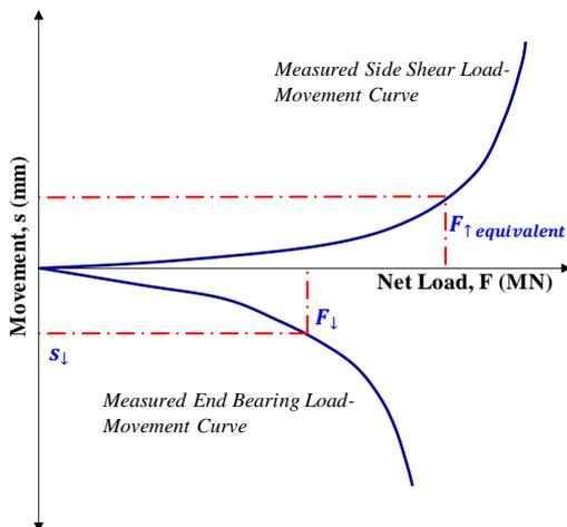
Figure 16 Upward and downward movement vs load curves
