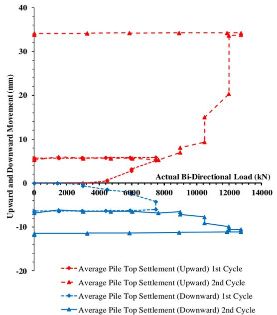
Figure 14 Upward and downward movement against applied load
