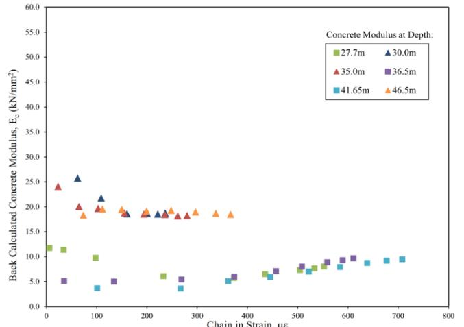
Figure 9 Back Calculated Concrete Modulus
