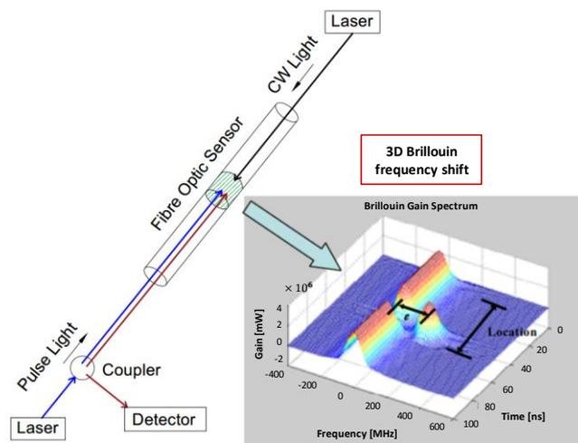
Figure 3 Principle of BOTDA sensor system (Lan *et al.*, 2012)
