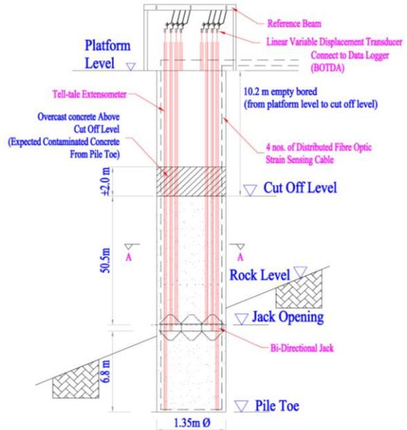
Figure 7 Schematic diagram of the BDSLT setup
