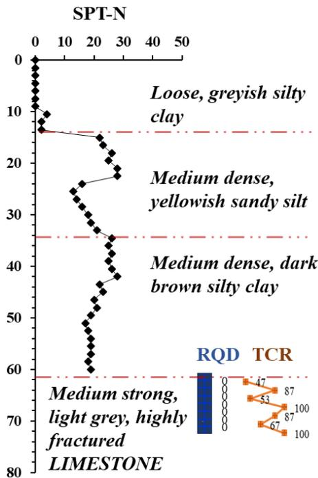
Figure 6 Geological Information of pile location
