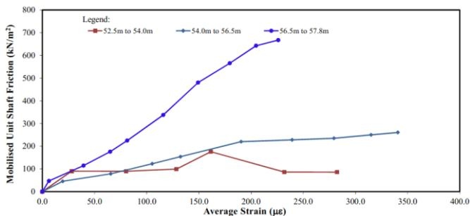
Figure 12 Mobilized Unit Shaft Friction (Lower Pile Section) against Average Strain
