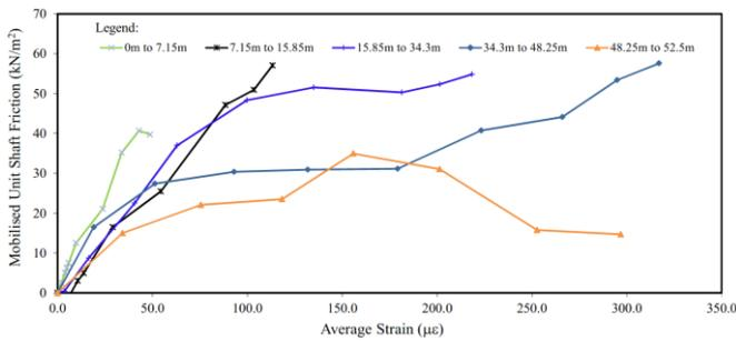
Figure 11 Mobilized Unit Shaft Friction (Upper Pile Section) against Average Strain
