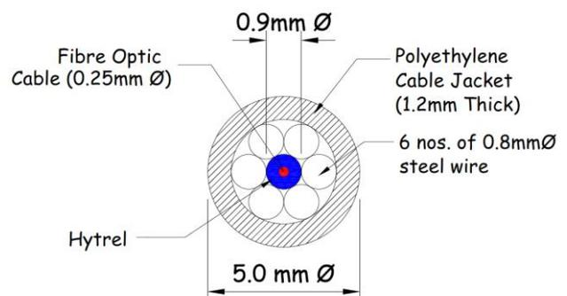
Figure 5 Configuration of strain sensing optical cable
