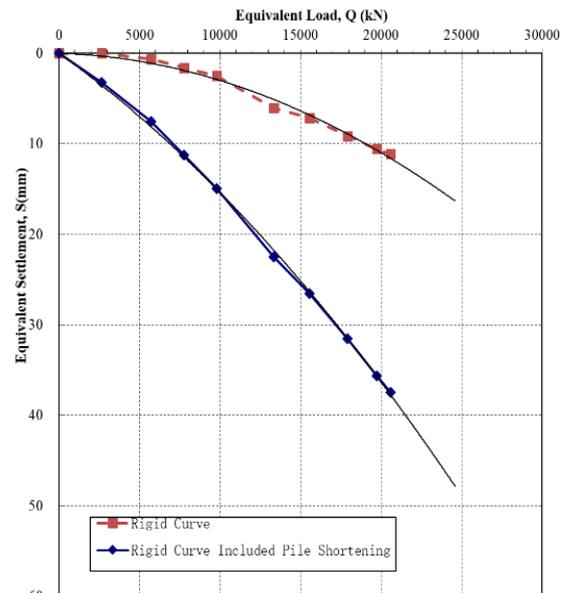
Figure 15 Equivalent top settlement curve
