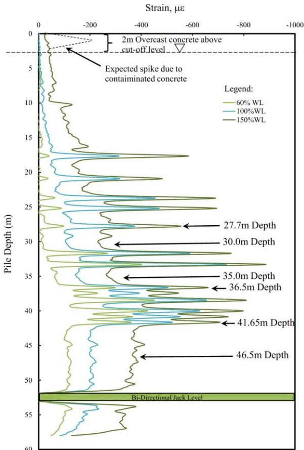
Figure 8 Change in strain along the pile during BDSLT
