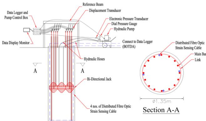
Figure 2 Typical Schematic Diagram of Bi-Directional Static Load Test
