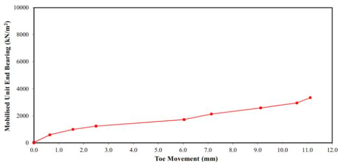
Figure 13 Mobilized Unit End Bearing against Toe Movement
