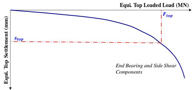
Figure 17 Conversion curve of top load versus movement
