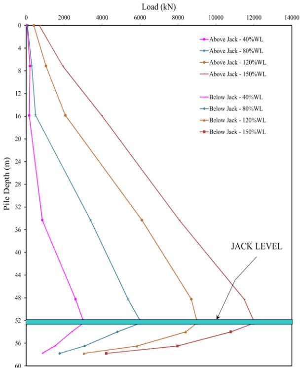
Figure 10 Load distribution along test pile
