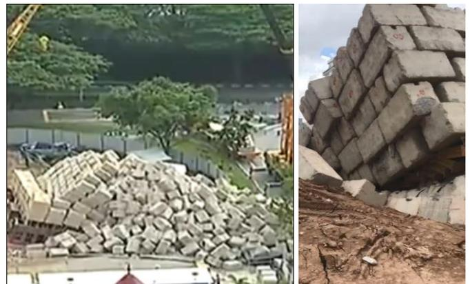
Figure 1 Examples of MLT kentledge system failure
