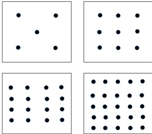
Figure 7 Helix piles with raft foundation distribution patterns plan
