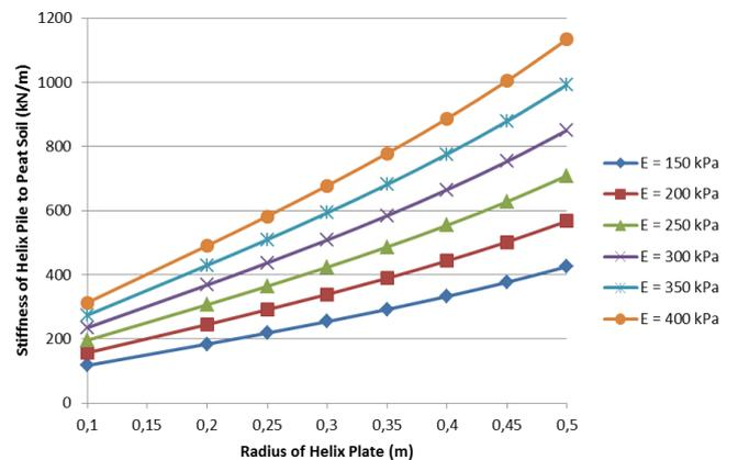
Figure 3 The effect of helice radius on the helix pile stiffness to peat soil
