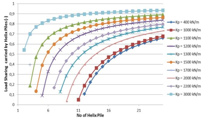
Figure 5 Load sharing ratio carried by helix piles at varies helix pile stiffness to peat soil
