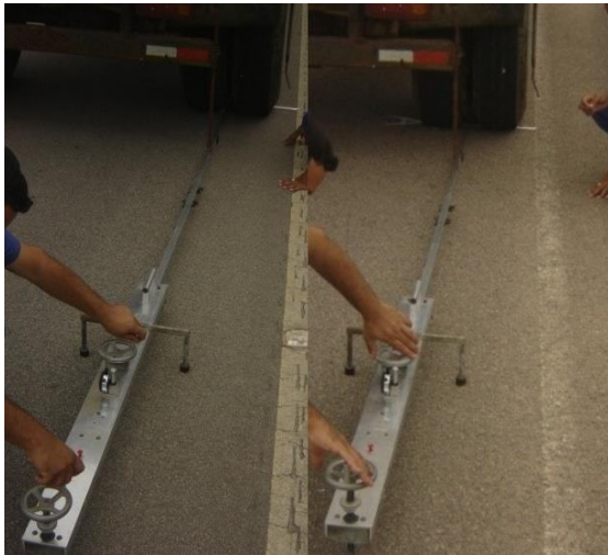
Figure 1 Benkelman Beam used
