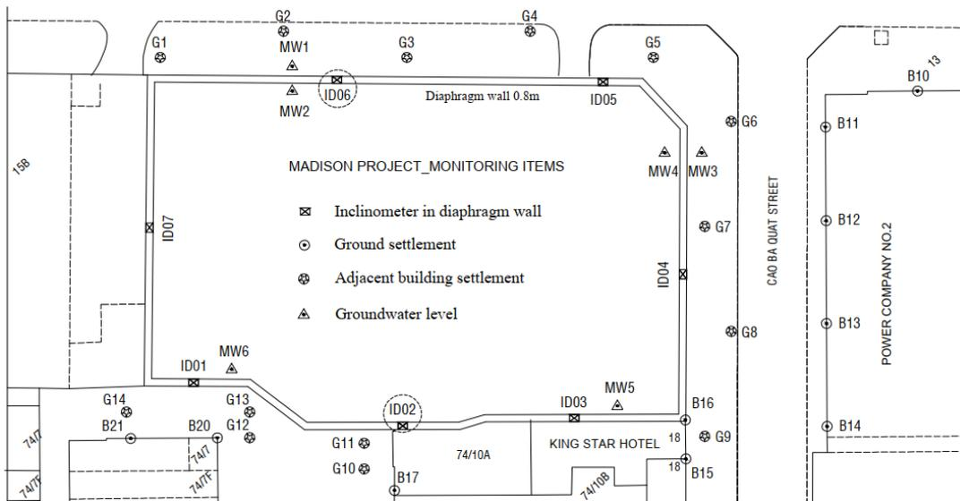
Figure 3 Arrangement of monitoring points (Case A)
