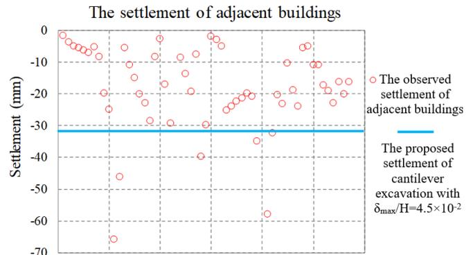
Figure 16 Comparison between observed and proposed settlement of Case H
