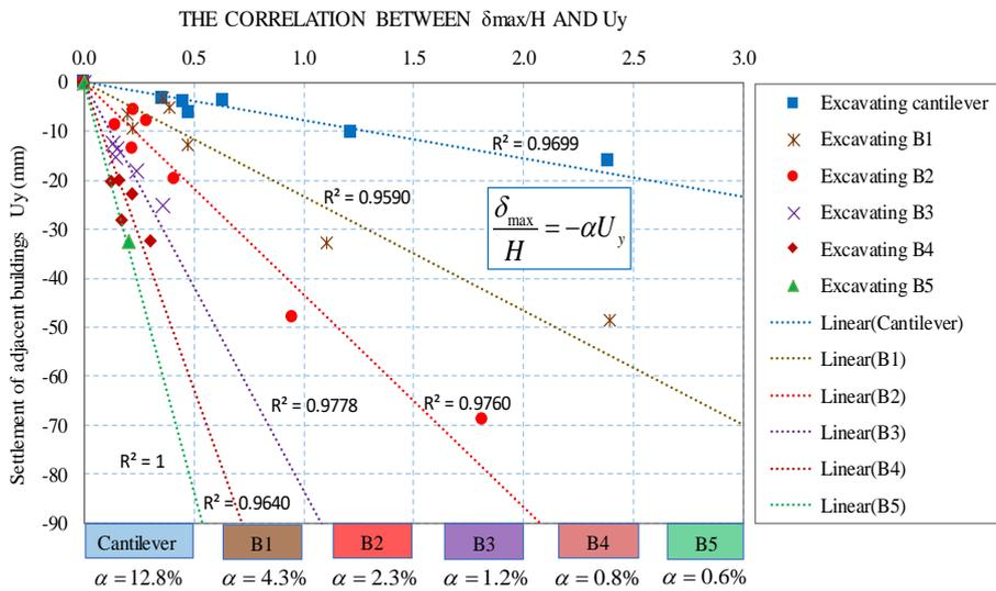
Max Lateral Wall Displacement / Excavation Depth,  $\delta_{max}/H$  (%)
