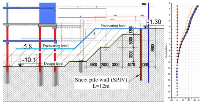
Figure 15 The real construction section and field data of lateral displacement of Case H
