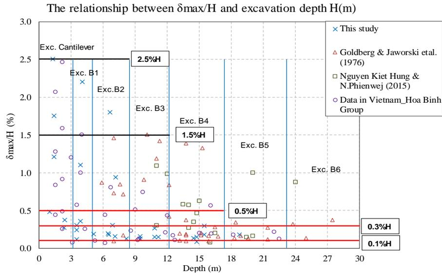
Figure 13 Relationship between  $\delta_{max}/H$  and excavation depth  $H(m)$
