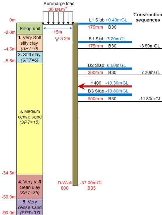
Figure 2 Construction section and soil profile of Case A
