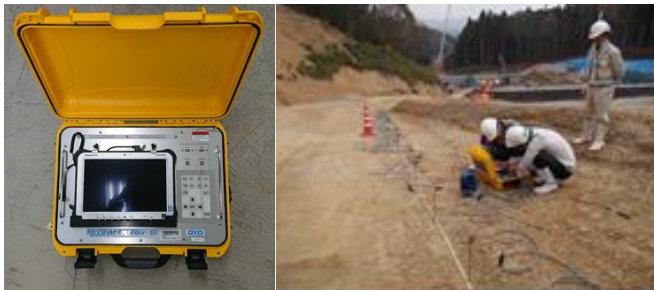
Figure 2 Electrical prospecting equipment and operation
