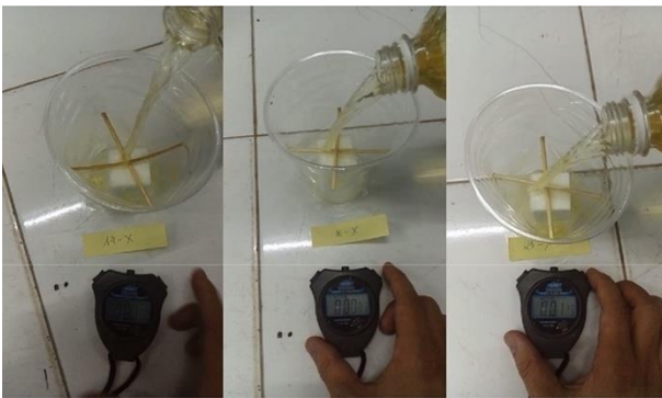
Figure 4 EPS Geofoam specimens submerging in diesel
