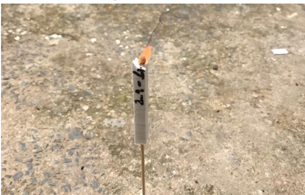
Figure 6 EPS Geofoam specimens contacting to fire
