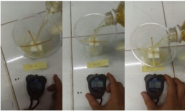
Figure 3 EPS Geofoam specimens contacting to gasoline
