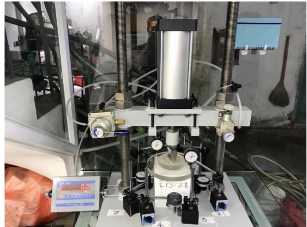
Figure 2 An instrument utilized for UCS tests in laboratory
