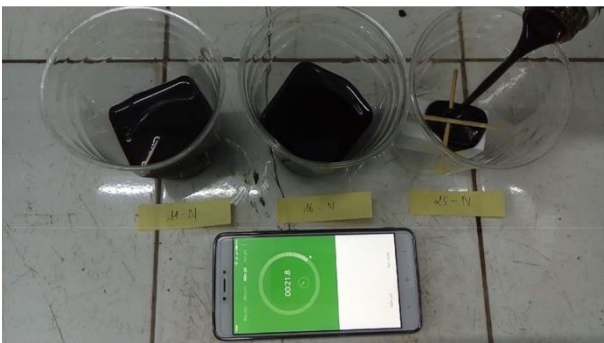
Figure 5 EPS Geofoam specimens immersing in a lubricant oil
