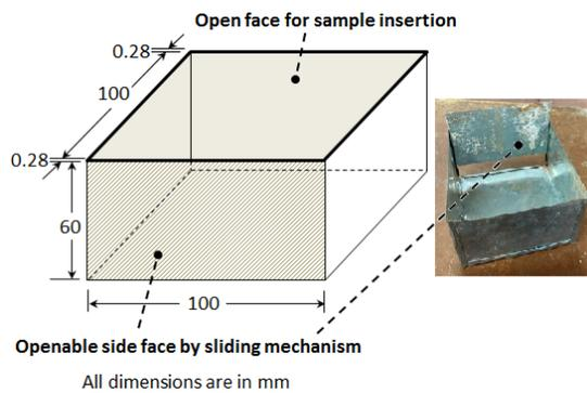
Figure 1 Details of the modified sampler box
