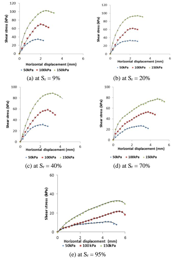
Figure 5 Results of direct shear tests on reconstituted samples under normal stress 50 kPa, 100 kPa, and 150 kPa
