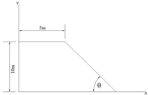
Figure 7 Typical slope model with slope inclination  $\theta$
