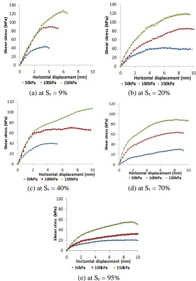
Figure 4 Results of direct shear tests on undisturbed samples under normal stress 50 kPa, 100 kPa, and 150 kPa
