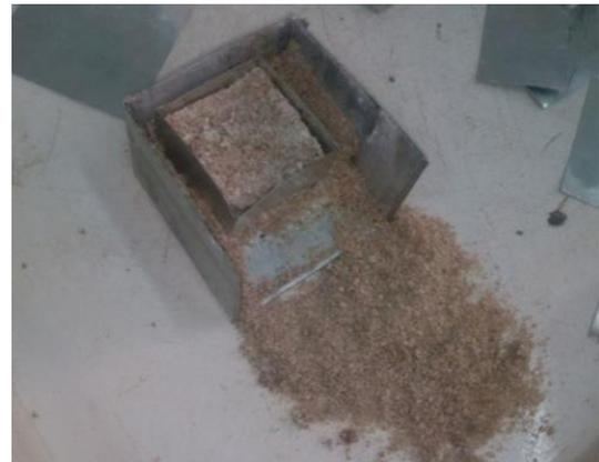
Figure 3 Extraction of undisturbed sample for direct shear test
