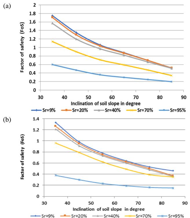
Figure 8 Decrease in FoS with Slope angle for different Sr%: (a) for undisturbed samples and (b) for remoulded samples
