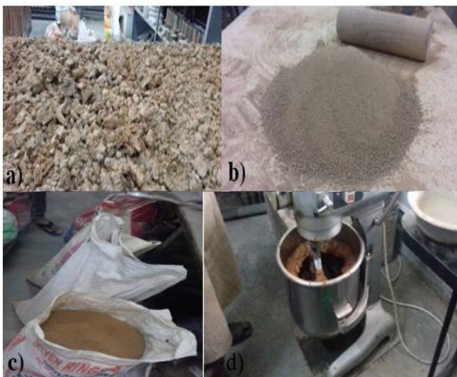
Figure 3 (a) The soft clay soil before oven-dry, (b) Soil after oven-dry (c) Dry sample in a bag, and (d) The mixing of sample to gain liquid limit
