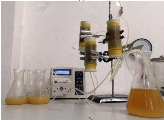
Figure 3 Test setup for microbial-reinforced: (a) Sketch of MICP reinforced procedure and (b) MICP reinforced in the lab
