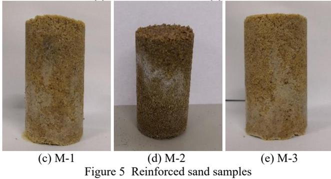
Figure 5 Reinforced sand samples
