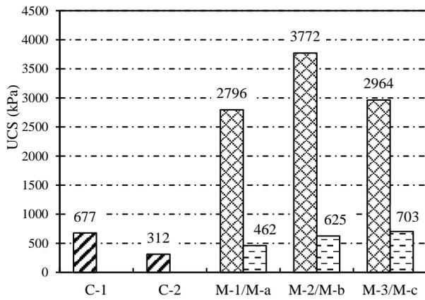
Figure 6 UCS of cement-treated and microbial-treated sands
