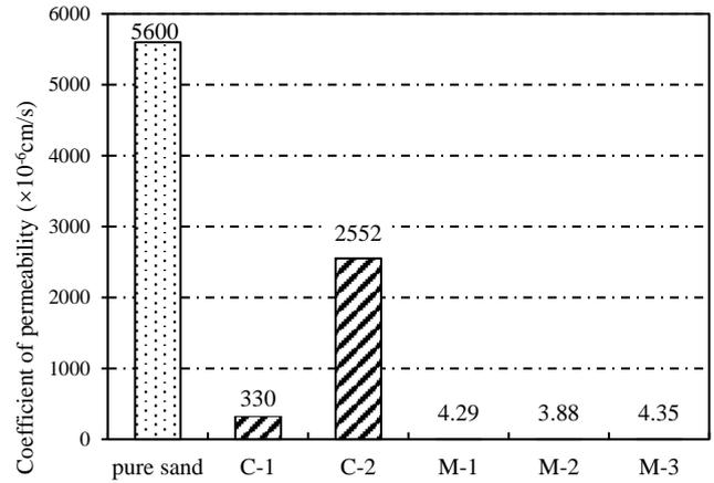
Figure 7 Permeability coefficients of pure and treated samples
