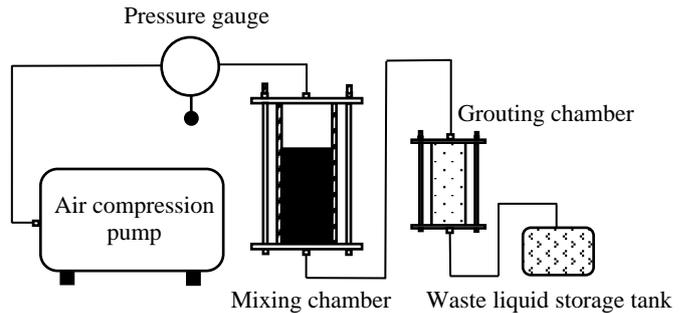
Figure 2 Schematic diagram of cement grouting (Bordier et al., 2000)
