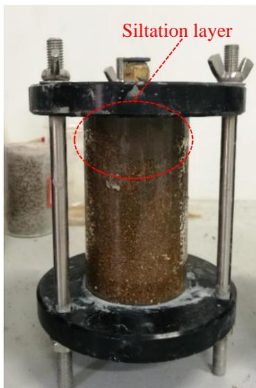
Figure 4 Channel blockage during cement grouting
