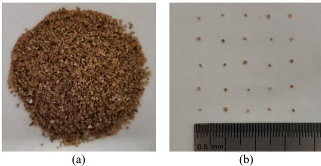
Figure 1 Sand sample used in this study: (a) Sand dune and (b) Sand particles
