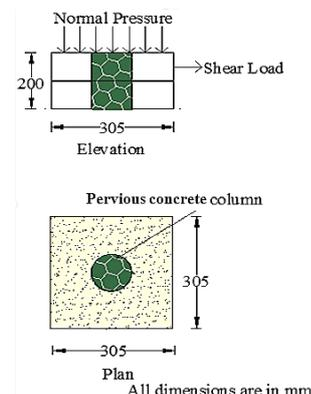
Figure 1(a) Direct shear test for pervious concrete column-treated ground
