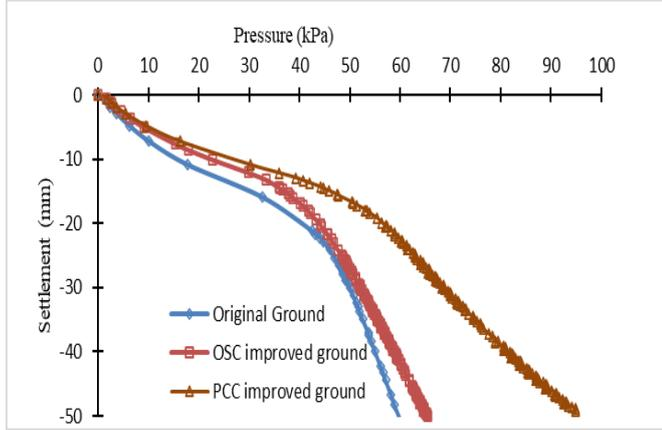
Figure 3(a) Impact of pervious concrete column (from large shear test model)
