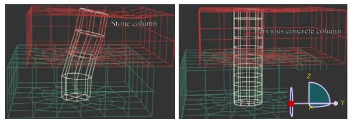
Figure 2(b) Deformed stone column and pervious concrete column after direct shear analysis
