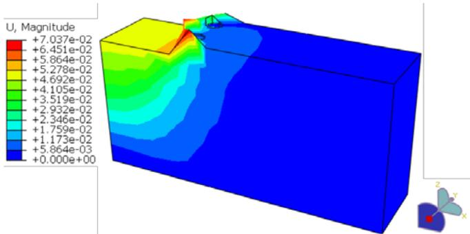
Figure 3(b) Deformed pervious concrete column treated ground with two columns from large shear test analysis
