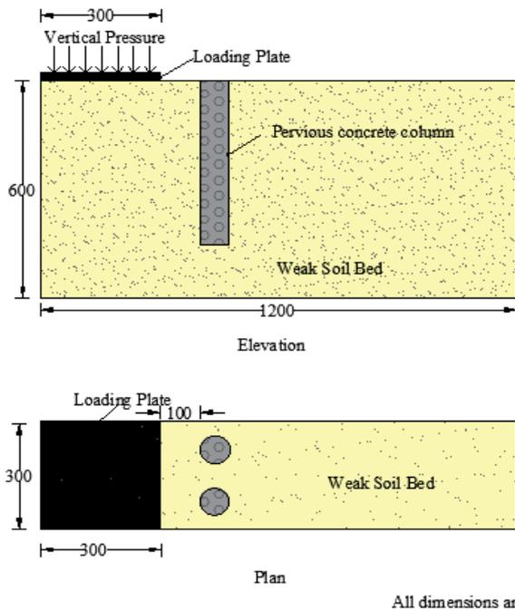
Figure 1(b) Large shear test model with two columns at 200 mm c/c arrangement
