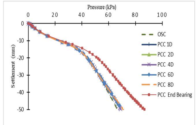
Figure 4 Impact of the depth of the pervious concrete column
