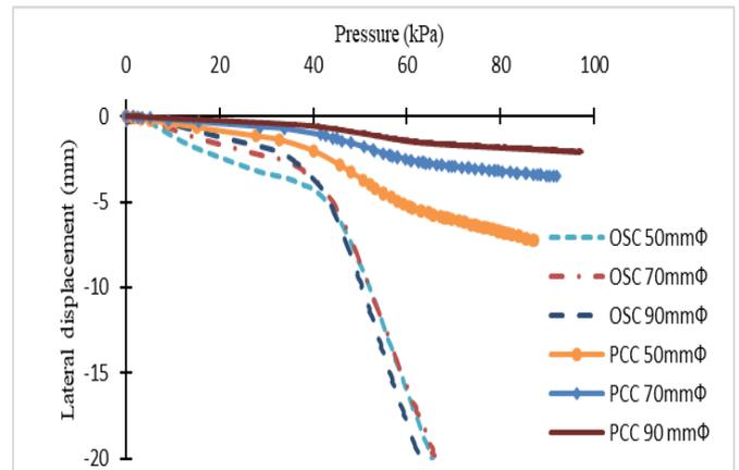
Figure 5 Pressure versus lateral deflection of the top end of the end-bearing columns
