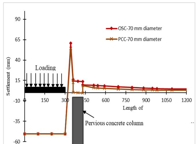
Figure 6 Heave profile observed for weak soil
