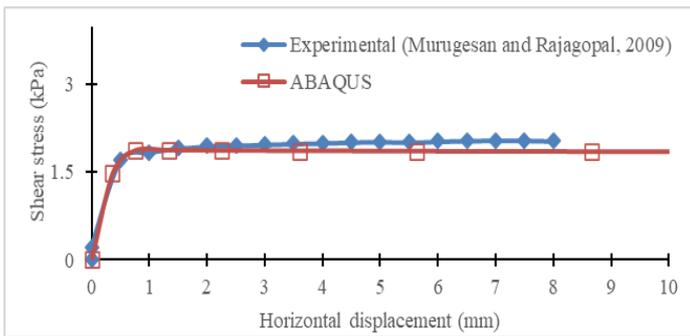
Figure 1(c) Validation of ABAQUS model.
