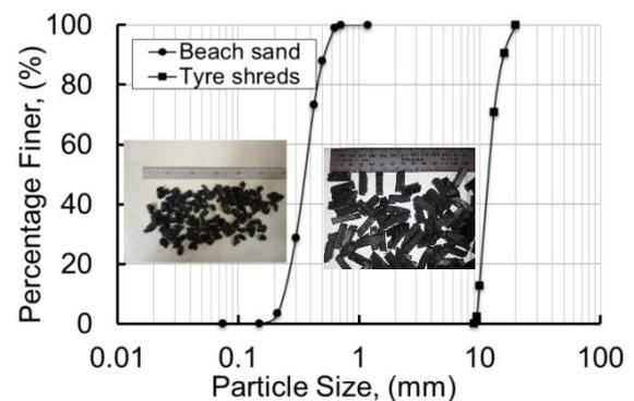
Figure 1 Particle size distributions of Sand and Tyre Shreds (inset: tyre shred and tyre chips)
