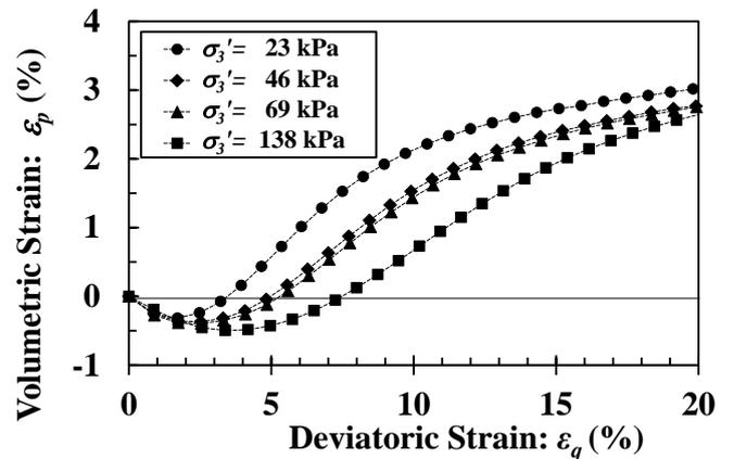
Figure 10 Variation of volumetric strain with deviatoric strain for different confining pressure (after Mashiri et al., 2015a)
