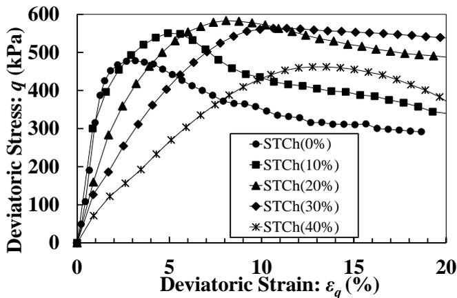
Figure 7 Variation of deviator stress with deviatoric strain for different proportion of TCh (after Mashiri et al., 2015a)
