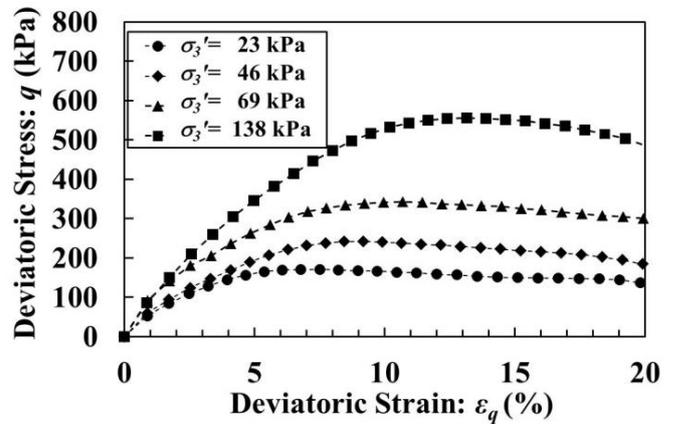
Figure 9 Variation of deviatoric stress with deviatoric strain for different confining pressure (after Mashiri et al., 2015a)
