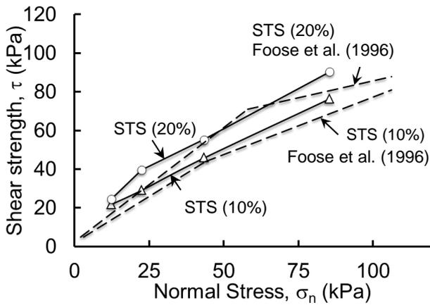
Figure 6 Variation of shear stress with normal stress for sand-tyre shred (STS) mixtures (after Vinod et al., 2015)
