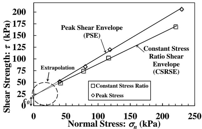
Figure 11 Typical shear envelope for STCh mixtures (after Mashiri et al., 2015a).
