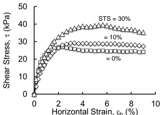
Figure 2 Variation of shear stress with horizontal strain (after Vinod et al., 2015)
