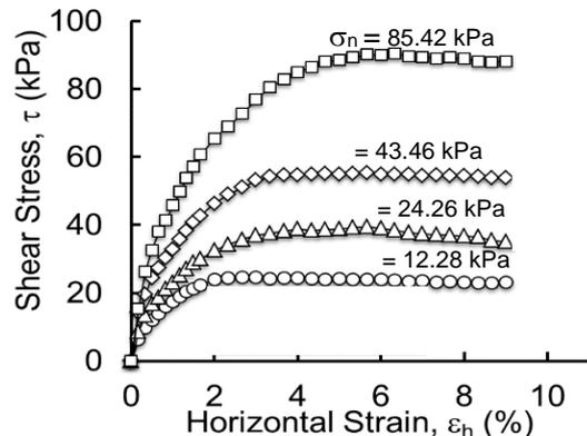
Figure 4 Variation of shear stress with horizontal strain for different confining pressure (after Vinod et al., 2015)
