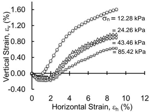
Figure 5 Variation of vertical strain with horizontal strain for different confining pressure (after Vinod et al., 2015)
