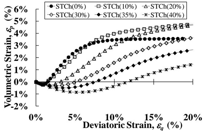
Figure 8 Variation of volumetric strain with deviatoric strain for different proportion of TCh (after Mashiri et al., 2015a)
