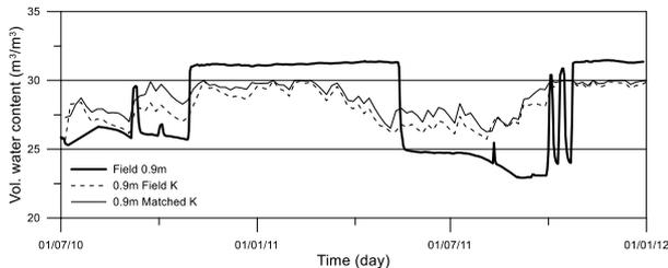
Figure 14 Measured and calculated VWC at 0.9 m depth at the crest location
