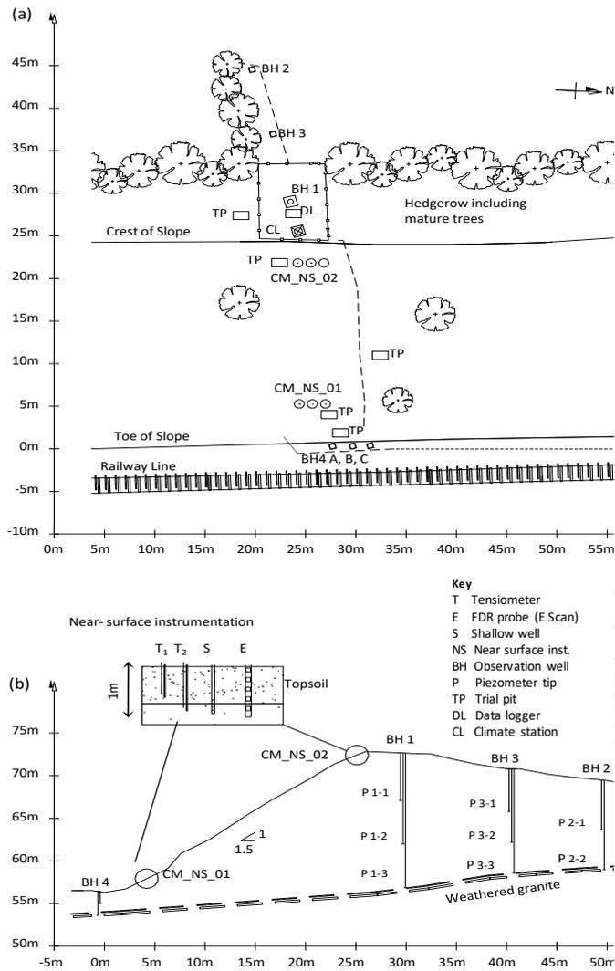
Figure 1 The Craigmore research site plan view and cross-section including instrumentation details (McLernon, 2014)
