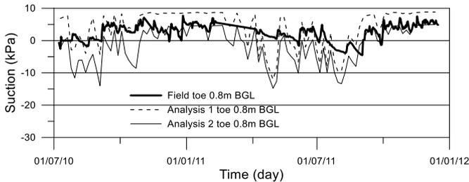
Figure 12 Measured and calculated suctions at the toe location 0.8 m BGL
