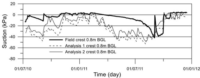
Figure 13 Measured and calculated soil suctions at the crest location 0.8 m BGL
