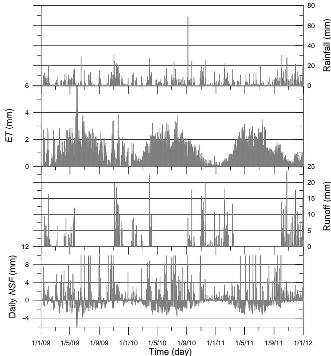
Figure 8 Recorded rainfall, calculated  $ET$ , surface runoff and  $NSF$  (Analysis 2) for Craigmore research site (2009-2011)
