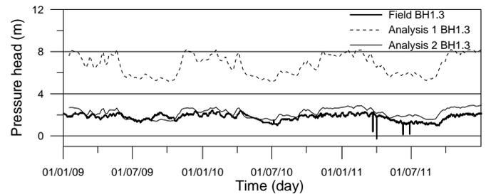
Figure 11 Measured and calculated pwp head for BH1.3 from two different analyses
