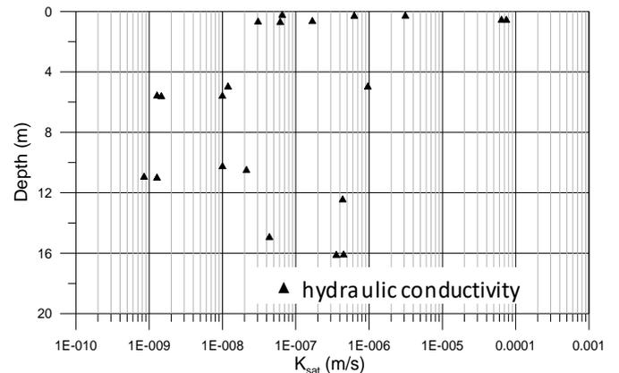
Figure 3 Saturated hydraulic conductivity determined from different field tests (Carse, 2014)
