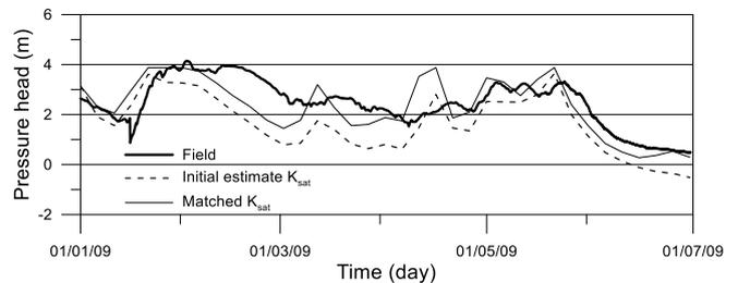
Figure 6  $K_{sat}$  estimation trial plots for Craigmore cutting at BH1.1
