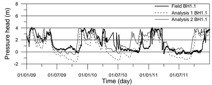
Figure 9 Measured and calculated pwp heads for BH1.1 from two different analyses
