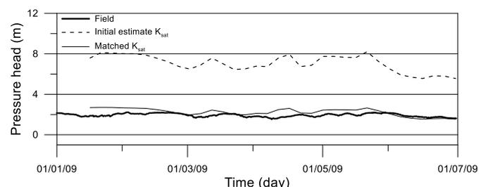
Figure 7  $K_{sat}$  estimation trial plots for Craigmore cutting at BH1.3
