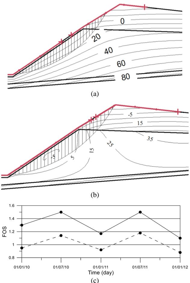
Figure 15 Pwp distribution (contour labels are in kPa) in Craigmore cutting on 1 January 2014: (a) Analysis 1, (b) Analysis 2, and (c) FOS changes with time in the two analyses
