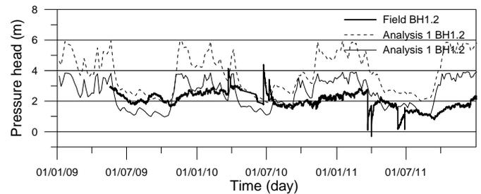
Figure 10 Measured and calculated pwp head for BH1.2 from two different analyses
