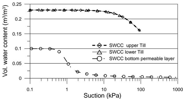
Figure 5 SWCCs used for material models used in Craigmore cutting analyses (McLernon, 2014)
