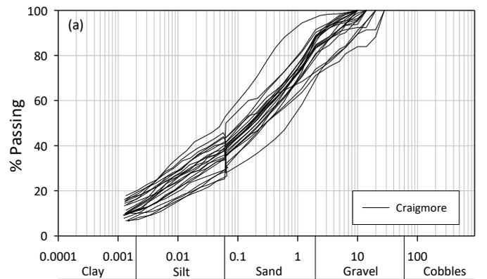
Figure 2 Particle size distribution for samples collected from different depths at Craigmore cutting (McLernon, 2014)
