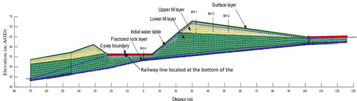
Figure 4 Discretized geometry used for the Craigmore cutting analyses
