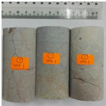
Figure 3 The three rock cores from locality 1 used for the Acoustic Velocity test and UCS test
