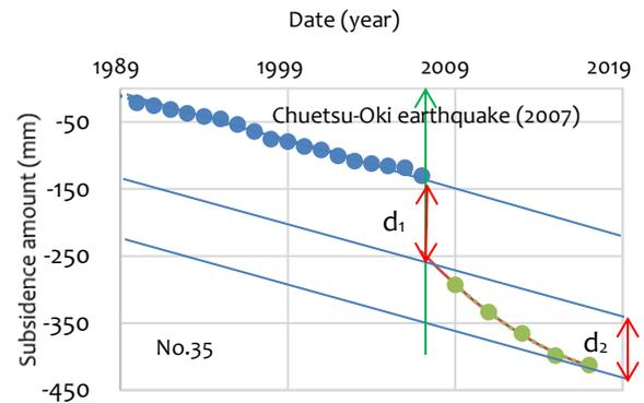
Figure 9 Typical examples of recorded land subsidence and time relationship (dune)
