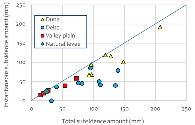
Figure 12 Instantaneous subsidence amounts and terrain classification
