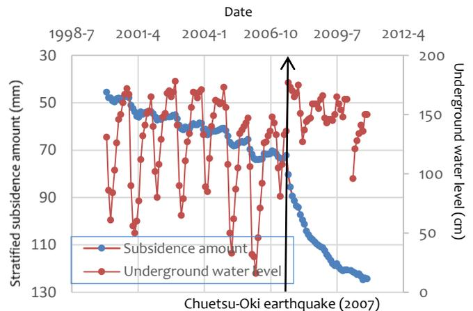
Figure 2 Stratified subsidence of clayey layer at Shimbashi
