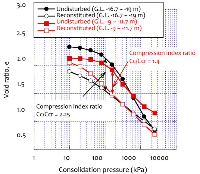
Figure 15 Compression characteristics of marine clay in undisturbed and reconstituted conditions
