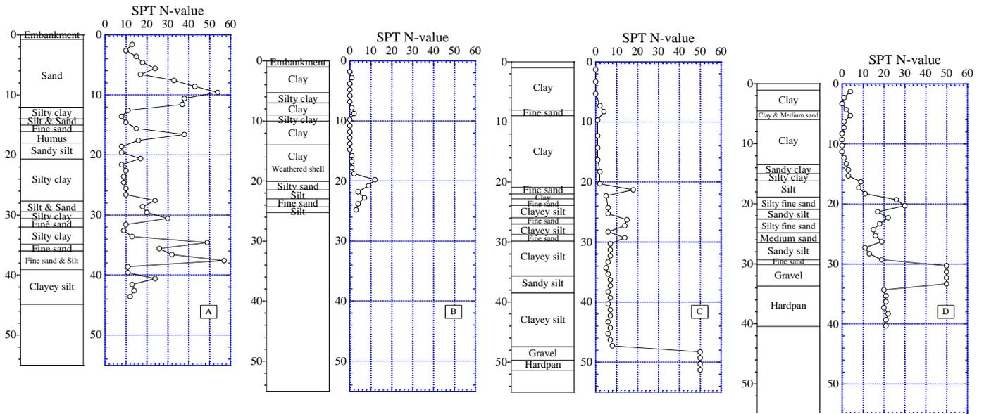
Figure 6 Geological columns and SPT-N values at four sites in typical terrain classification: (a) City hall in dune, (b) Shimbashi-A in delta, (c) Shimbashi-B in delta, and (d) Johtoh in valley plain.
