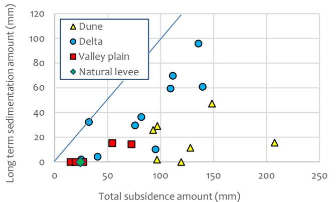
Figure 13 Long-term subsidence amounts and terrain classification
