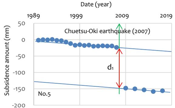
Figure 8 Typical examples of recorded land subsidence and time relationship (dune)
