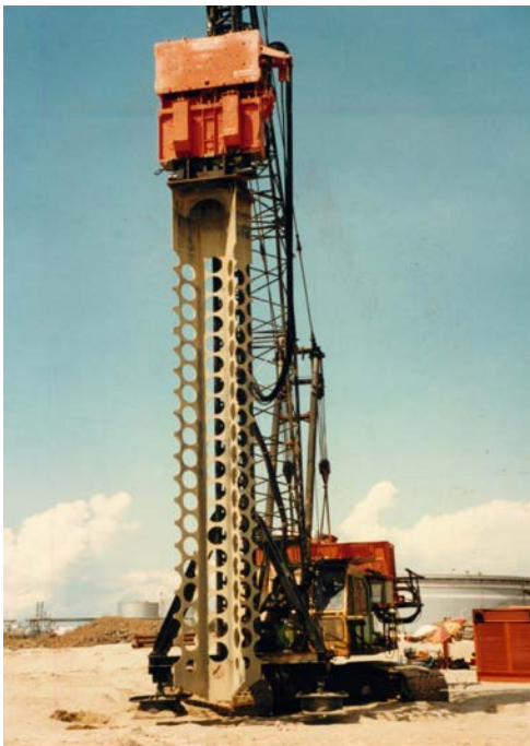
Figure 3 DVVC machine with a variable frequency vibrator and flexible double-Y probe
