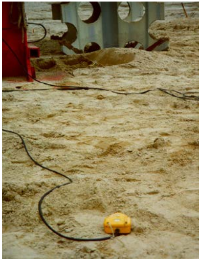
Figure 7 Tri-axial geophone for measurement of resonance frequency at 4 m distance from compaction probe
