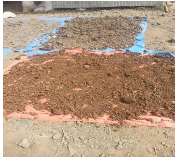
Figure 3 Air drying of samples and sample preparation for the test
