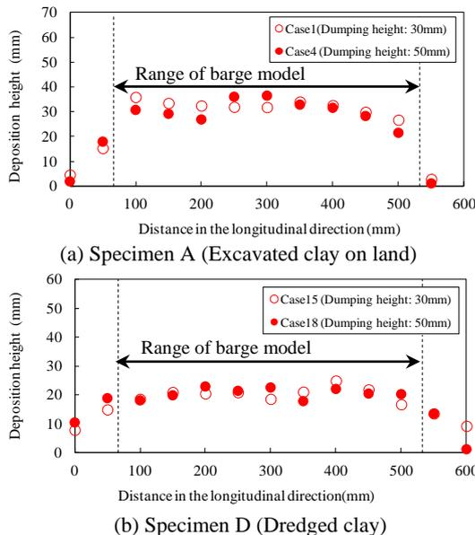
Figure 11 Comparison of deposition shapes for the cases with different dumping heights
