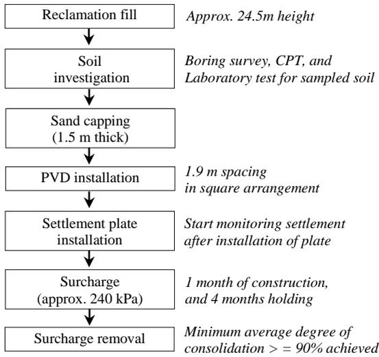
Figure 18 Work sequences in reclamation and ground Improvement
