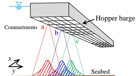
(a) Deposition shape of soil dumped from each compartment
