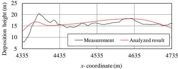
Figure 16 Comparison of measurement and analyzed results on deposition height
