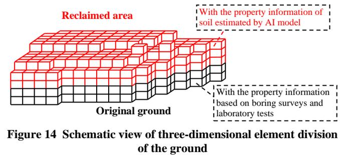
Figure 14 Schematic view of three-dimensional element division of the ground
