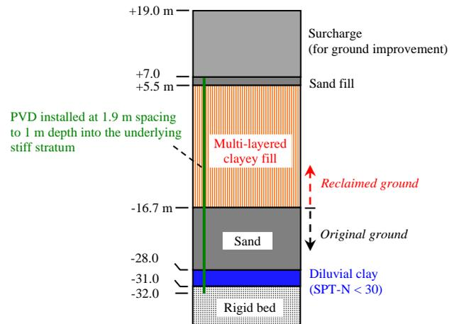
Figure 21 Soil model in the reclamation area
