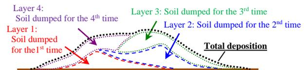
(b) Deposition shape and internal layers of soils formed
