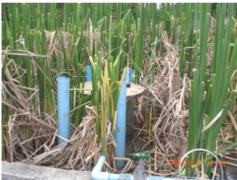
Figure 10 Close flux chamber in operation
