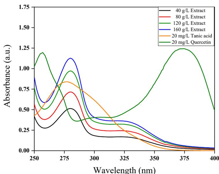
**Figure 2.** UV-Vis spectra of extract dyes from mangosteen leaves at different concentrations.
