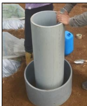
Figure 4 Double ring infiltration test.
