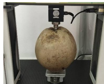
Figure 2 Quasi-static compression test by Universal Testing Machine.
