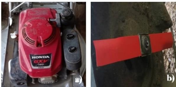
Figure 6 a) 5.5 hp engine b) grass cutting blade.
