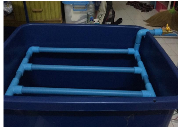
Figure 3 Water spray system structure assembled.
