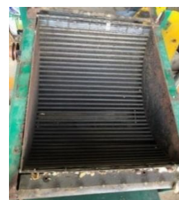
Figure 6 The steel-bar sieve.
