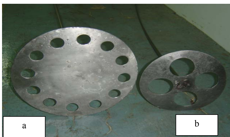
Figure 6 Different manual plungers; a) ISO standard and b) KU design.
