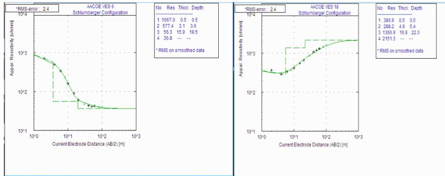
Figure 4. Typical sounding curves (VES 6 and 18) in the study area
