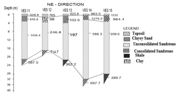
Figure 7. Geoelectric section profiles three
