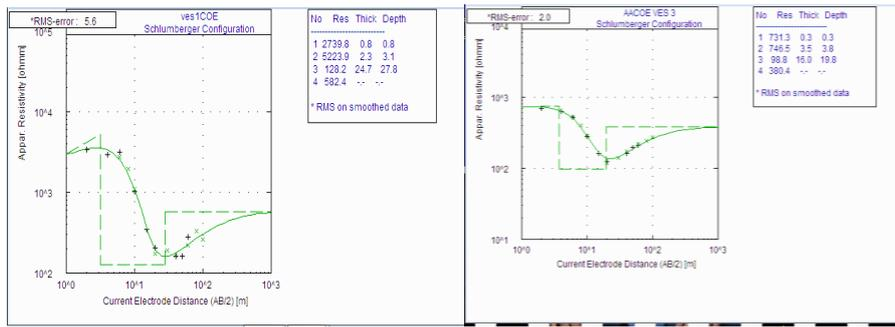
Figure 3. Typical sounding curves (VES 1 and 3) in the study area
