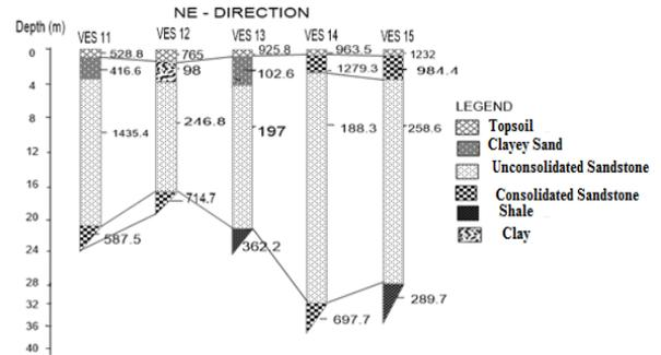
Figure 6. Geoelectric section along profile two
