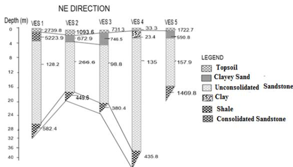
Figure 5. Geoelectric section profiles one
