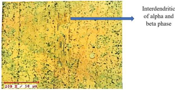
Figure 10. Microstructure image of SMAs
