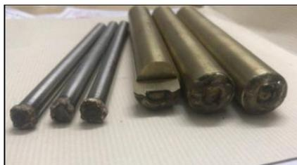
Figure 5. Welded joints after testing (Set-2)
