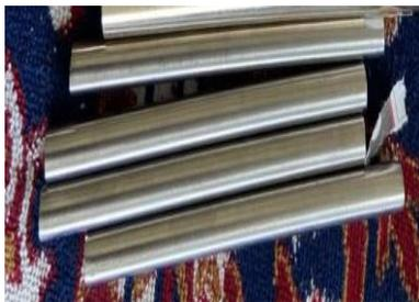
Figure 3. Iron based SMA (Fe Mn Si Cr Ni)
