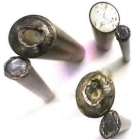
Figure 4. Welded joints after testing (Set-1)
