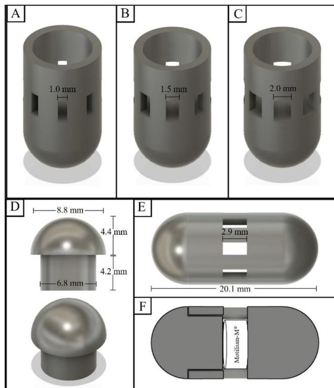
**Figure 1** Illustration of HPD; the dimension of the bodies with a hole width of (A) 1.0 mm, (B) 1.5 mm, and (C) 2.0 mm. (D) The dimension of the cap. (E) The whole device's dimension and (F) the vertical cut view of HPD shows a chamber area containing a Motilium-M<sup>®</sup> tablet.
