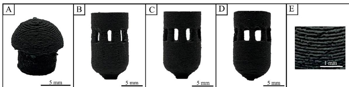
**Figure 2** The morphology of HPD. (A) The cap of HPD and the bodies of HPD with different hole widths (B) 1.0 mm, (C) 1.5 mm, and (D) 2.0 mm), and (E) the enlarged image of HPD.
