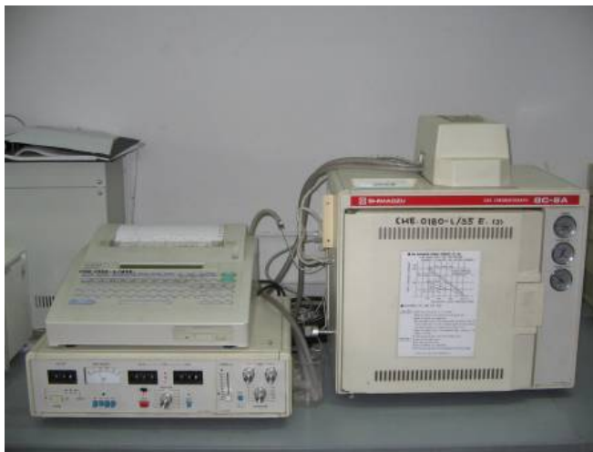
Figure 14 Shimadzu gas chromatograph equipped with thermal conductivity detector and chromatopac data processor.
