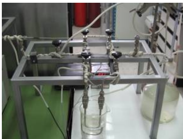
Figure 13 Heated sampling valve and U-tube cooling trap connecting to quick release valves.
