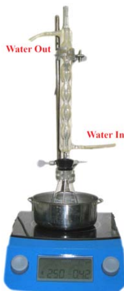
Figure 16 The setup of equipment for hydrolysis and condensation reactions.
