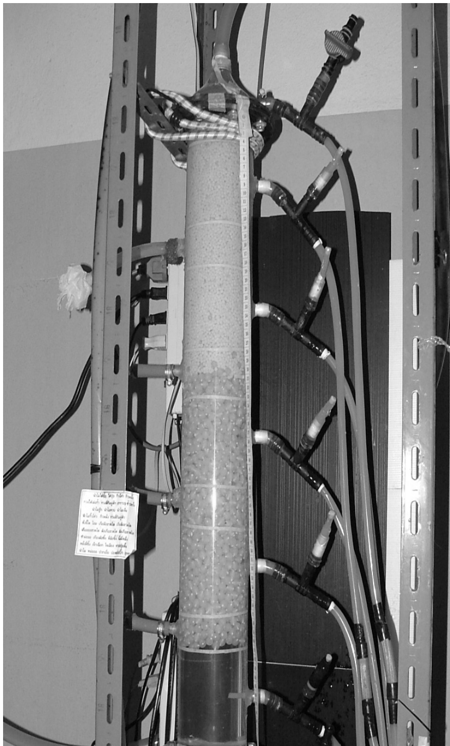
Figure 6 Floating plastic media flocculator column with 3-mm and 10-mm media sizes
