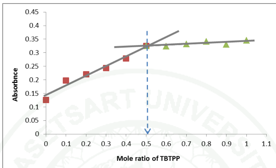
Figure 42 The mole ratio plot of complex between TBTPP and \text{Hg}^{2+} in ethanol.
