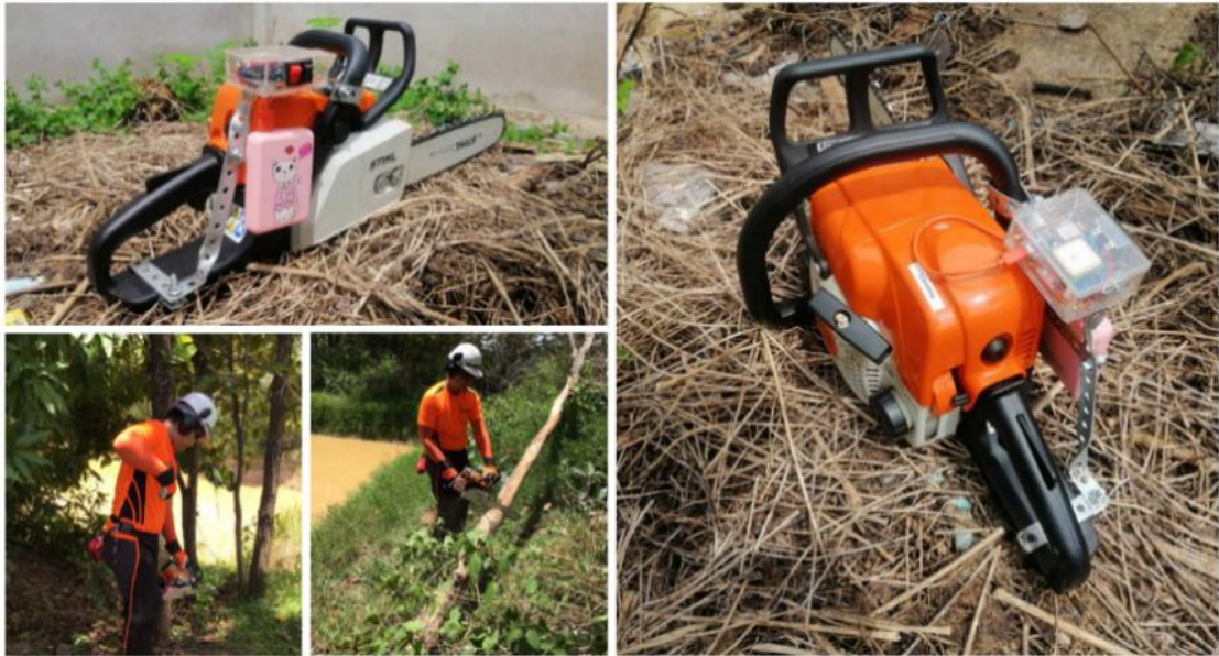
Figure 4 Installation and testing of the sensor.
