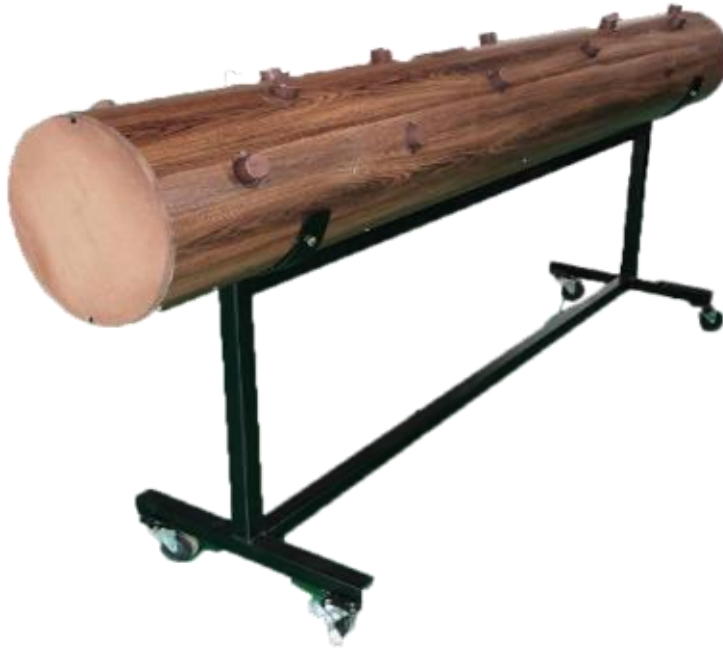
Figure 2 Developed model for practicing the chainsaw skills.
