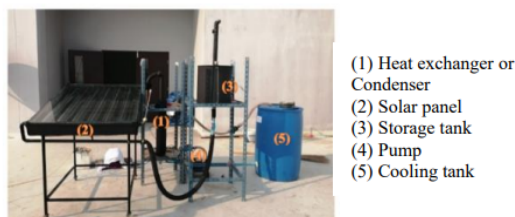
Fig. 2. Solar energy distillation system of citronella oil using bubble pump technique.
