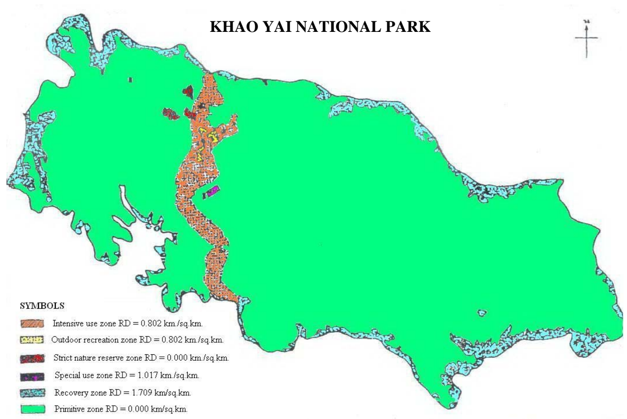
Figure 21 Forest roads density map in Khao Yai National Park classified by management zones.
