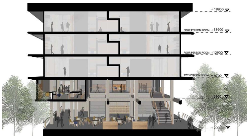
Figure 16 Application of the two keywords: shuffle and interlock. The double-height space of the canteen on the first floor encourages visual and physical connection to the co-working space on the second floor. The sleeping area of the living unit utilises the interlocking design. (Drawn by Matsombat, Saidarasamoot, Kiatsirikulthorn, and Poe Tun for INA242 class of 2/2020)
