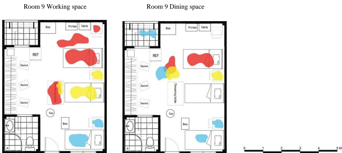
Figure 12 Unit Room 9 (three-persons room type) showing the working space and dining area. Colours are used to represent the three different users. (Source: Lumthaweepaisal, 2021)
