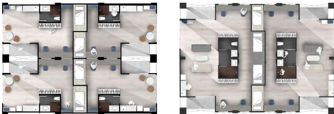
Figure 19 Furniture layout for the two-person room type (left) and four-person room type (right) showing the living environment and space organisation, improved from the existing dormitory conditions (Drawn by Matsombat, Saidarasamoot, Kiatsirikulthorn, and Poe Tun for INA242 class of 2/2020)
