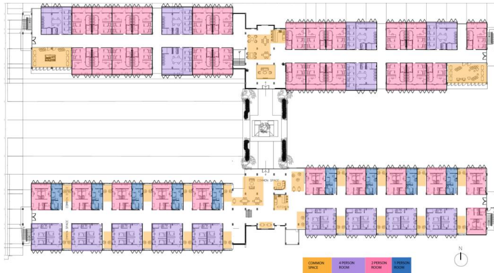
Figure 22 Second-floor plan of the building showing the cluster space with pocket communal facilities (Drawn by Petchsakaek, Mahasittichod, Chew, and Sornnarin for INA242 class of 2/2020)
