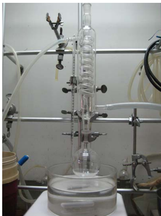
Figure 15 Apparatus for N-benzoyl-2-pyrrolidone synthesis.
