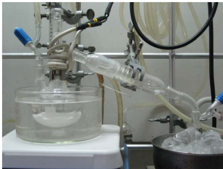
Figure 13 Apparatus for melt polycondensation of \gamma -aminobutyric acid and anionic ring-opening polymerization of dehydrated 2-pyrrolidone.
