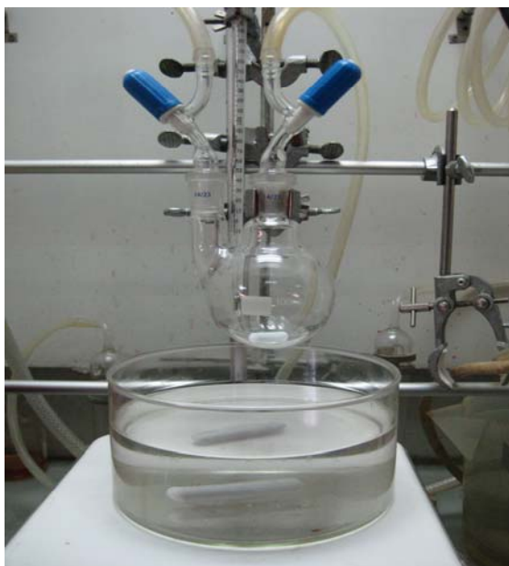
Figure 16 Apparatus for dehydration of 2-pyrrolidone.
