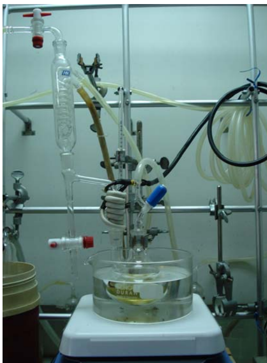
Figure 14 Azeotropic distillation apparatus with a Dean-Stark trap.
