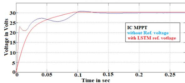
Figure 6. Converter output voltage with and without the utilization of LSTM  $V_{ref}$  value in IC MPPT
