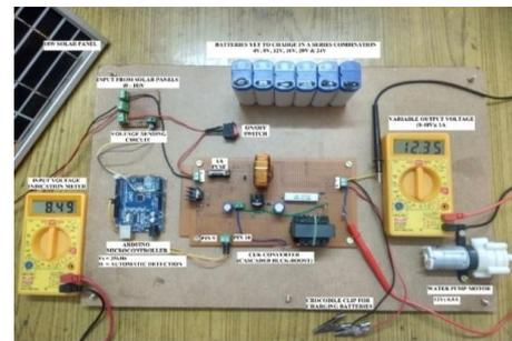
Figure 7. Overall hardware setup
