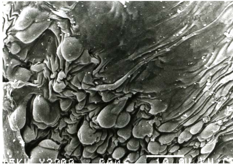
Figure 11 The surface of the nodular phase is deep fold and pleat.
