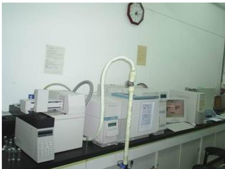
Appendix Figure B2 Gas chromatography-mass spectrometry (GC-MS) instrument.
