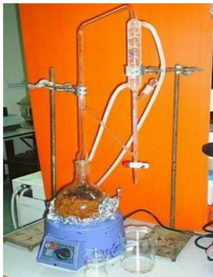
Appendix Figure B1 The Clevenger-type apparatus hydrodistillation extraction.
