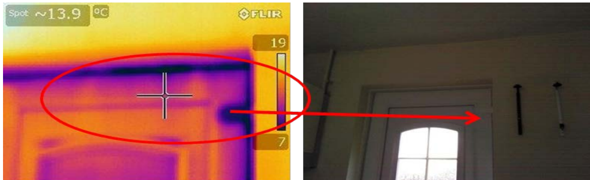
Figure 20: Defective seals on the top of the door profile
