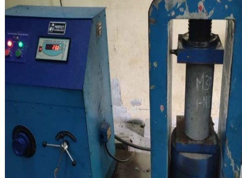
Figure 6: Cylinders Compressive Strength Test
