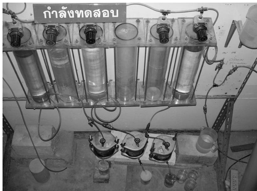
Figure 13 Permeability test apparatus
