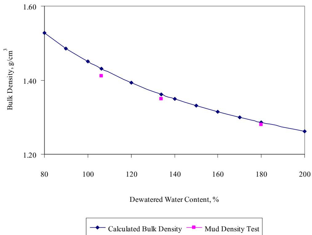
**Figure 20** Bulk densities and dewatered water content
