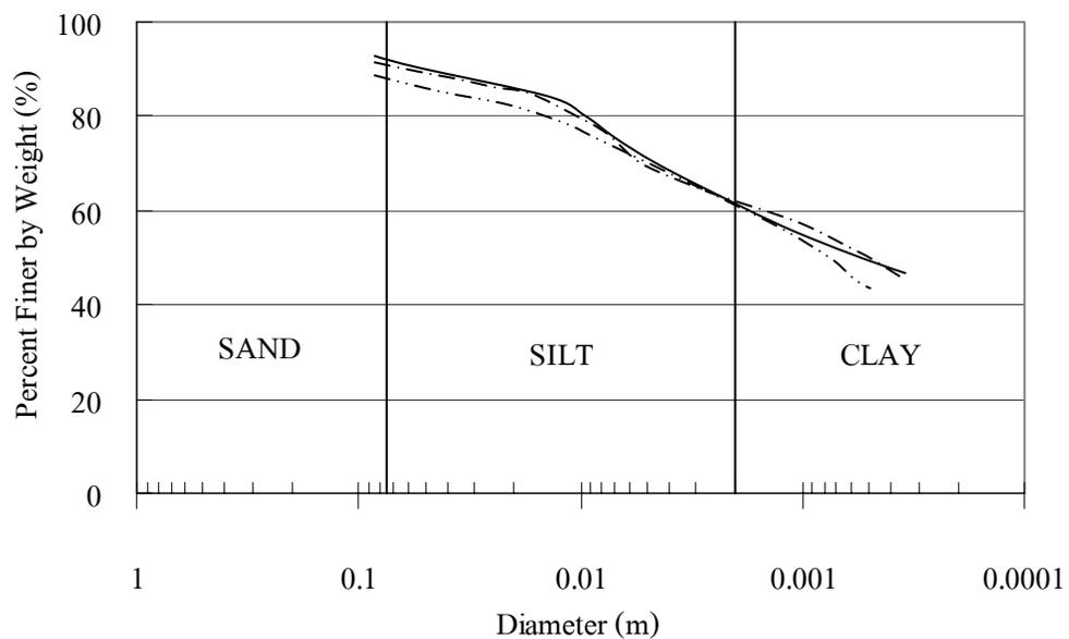
**Figure 17** Grain size distribution of untreated seabed dredged materials
