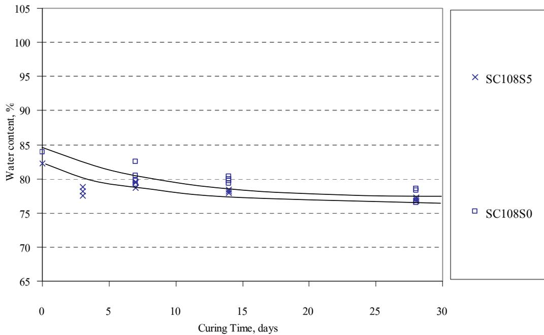
Figure 45 Curing water content of cement and sand mixed dredged materials with curing time (initial water content before mixing is 108.99%)
