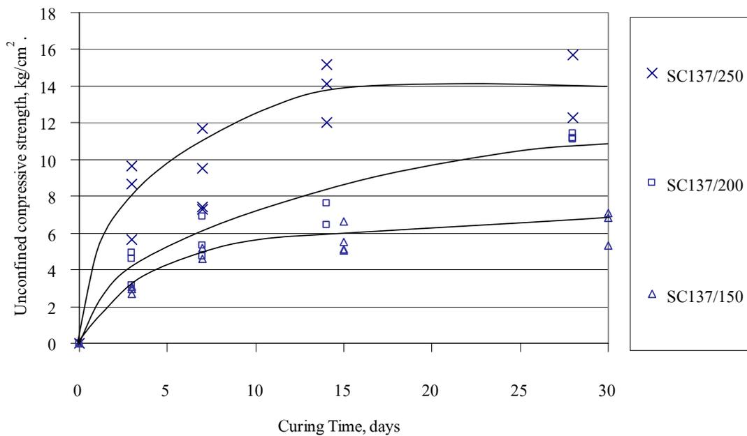
**Figure 22** Unconfined compressive strength of cement mixed dredged materials with curing time (initial water content before mixing was 137.87%)
