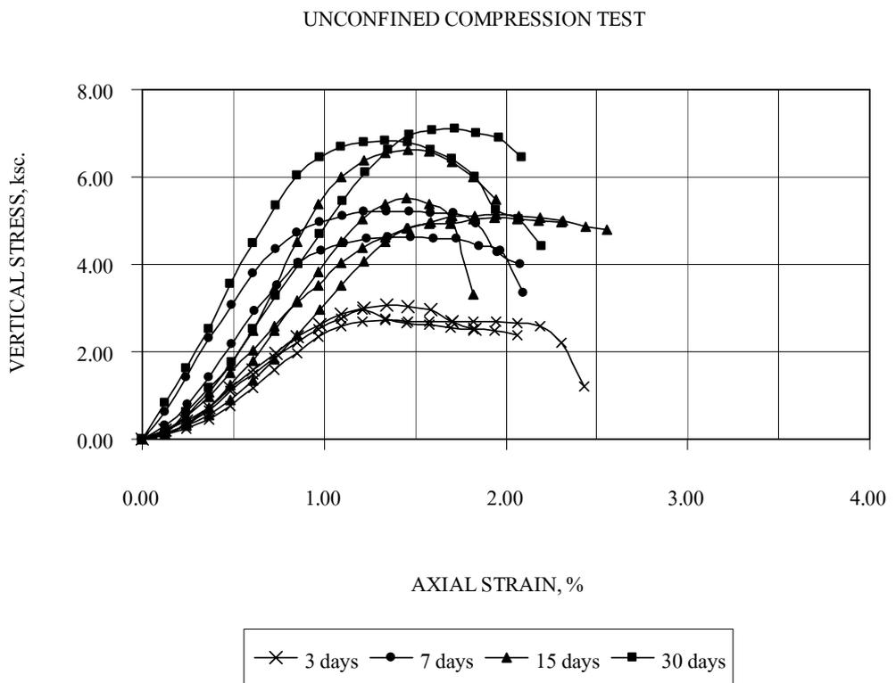
Appendix Figure 4 Stress-strain characteristics of SC137/150
