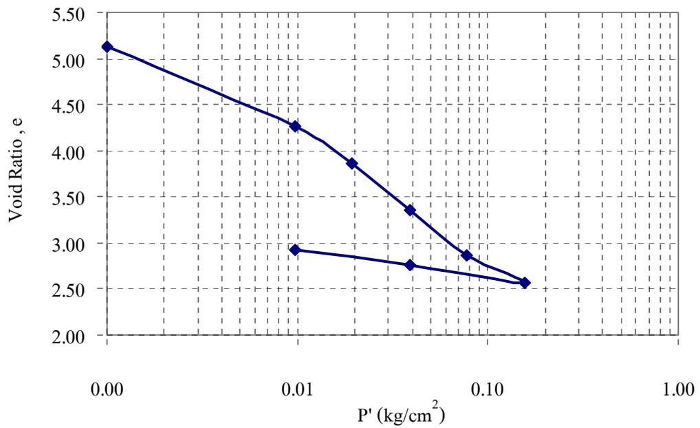
Figure 18 Void ratio and effective axial pressure relationship from consolidation test
