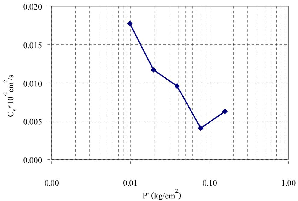
Figure 19 Coefficient of consolidation and effective axial pressure relationship from consolidation test
