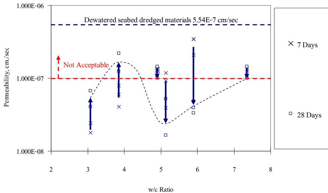
Figure 30 Permeability of cement mixed dredged materials with w/c ratio.
