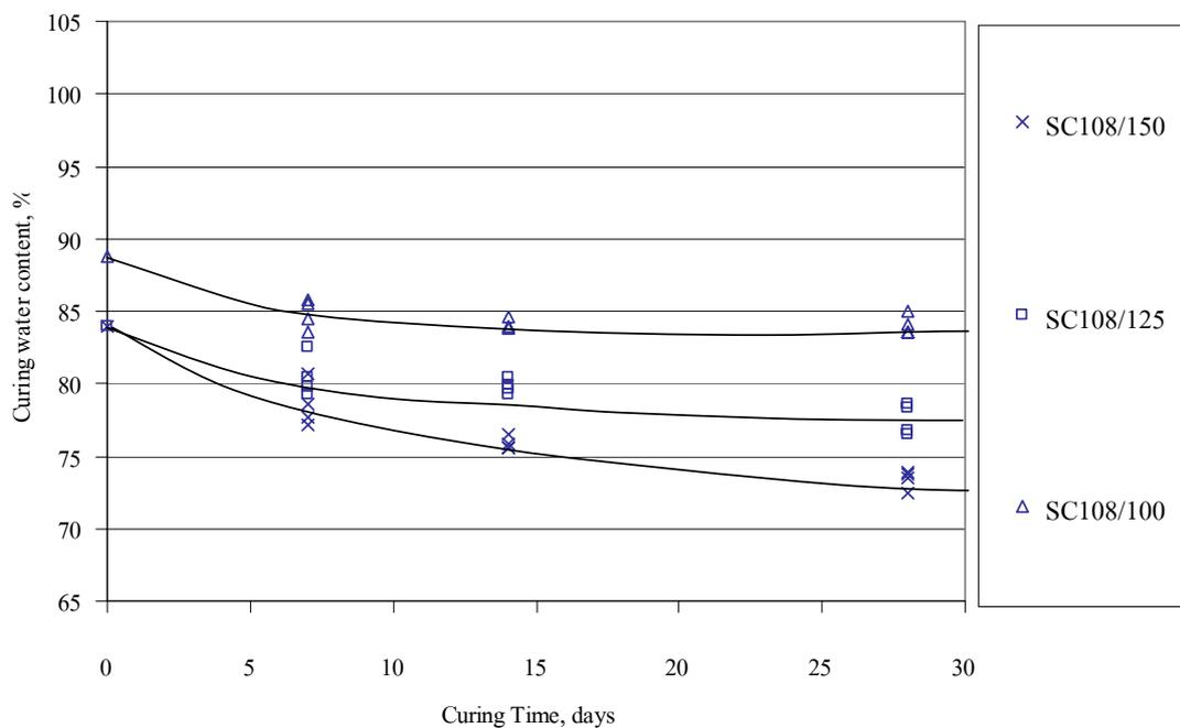
**Figure 33** Curing water content of cement mixed dredged materials with curing time (initial water content before mixing was 108.99 %)
