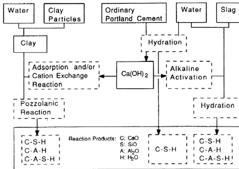
**Figure 4** Chemical reactions between untreated soil and hardening material
