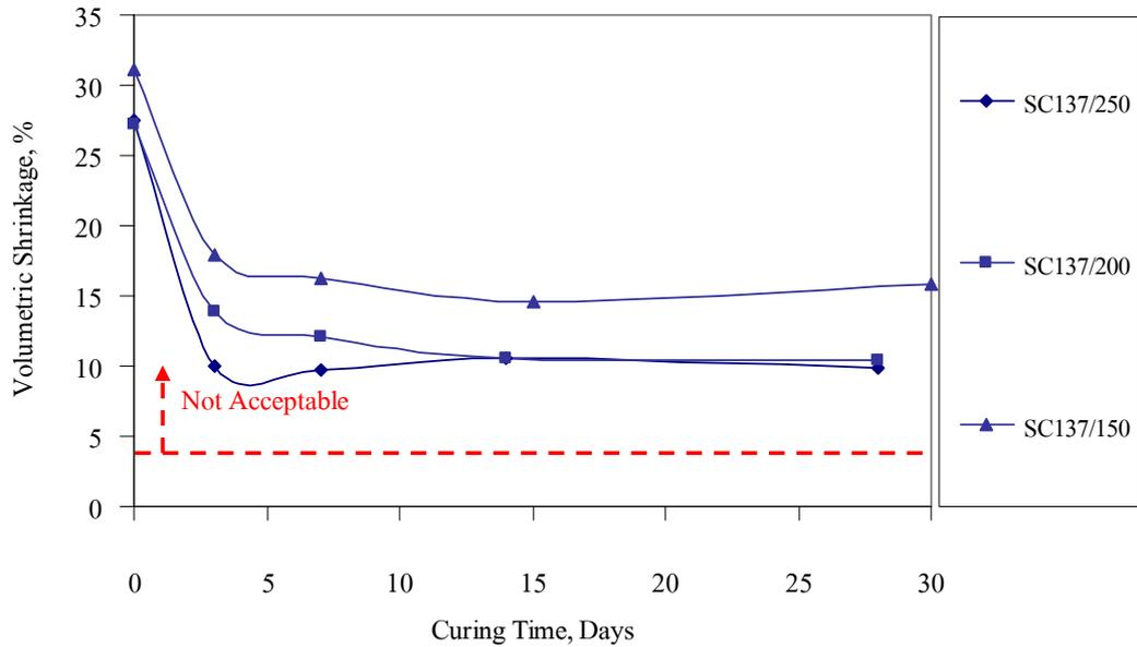
**Figure 32** Volumetric shrinkage of cement mixed dredged materials with curing time (initial water content before mixing was 137.87 %)
