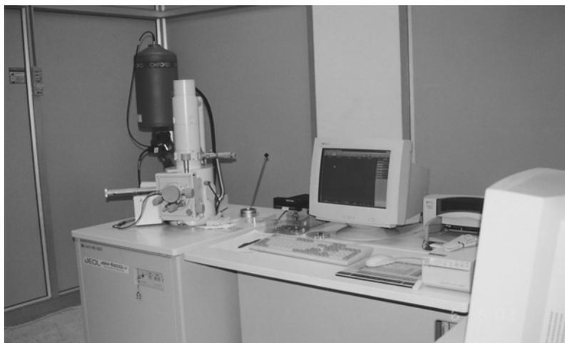
Figure 15 Scanning Electron Microscope (JEOL JSM-5600LV)
