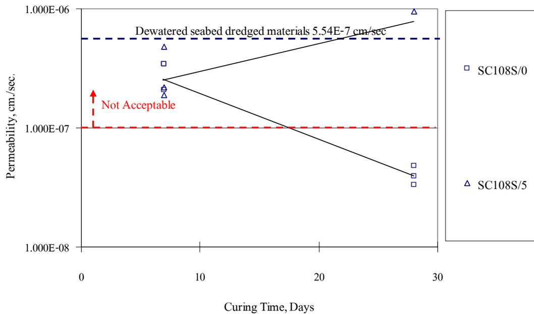
**Figure 43** Permeability of cement and sand mixed dredged materials (initial water content before mixing was 137.87%)
