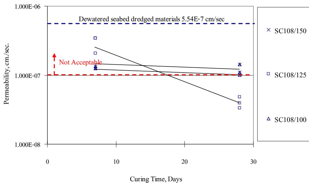
**Figure 26** Permeability of cement mixed dredged materials with curing time (initial water content before mixing was 108.99 %)
