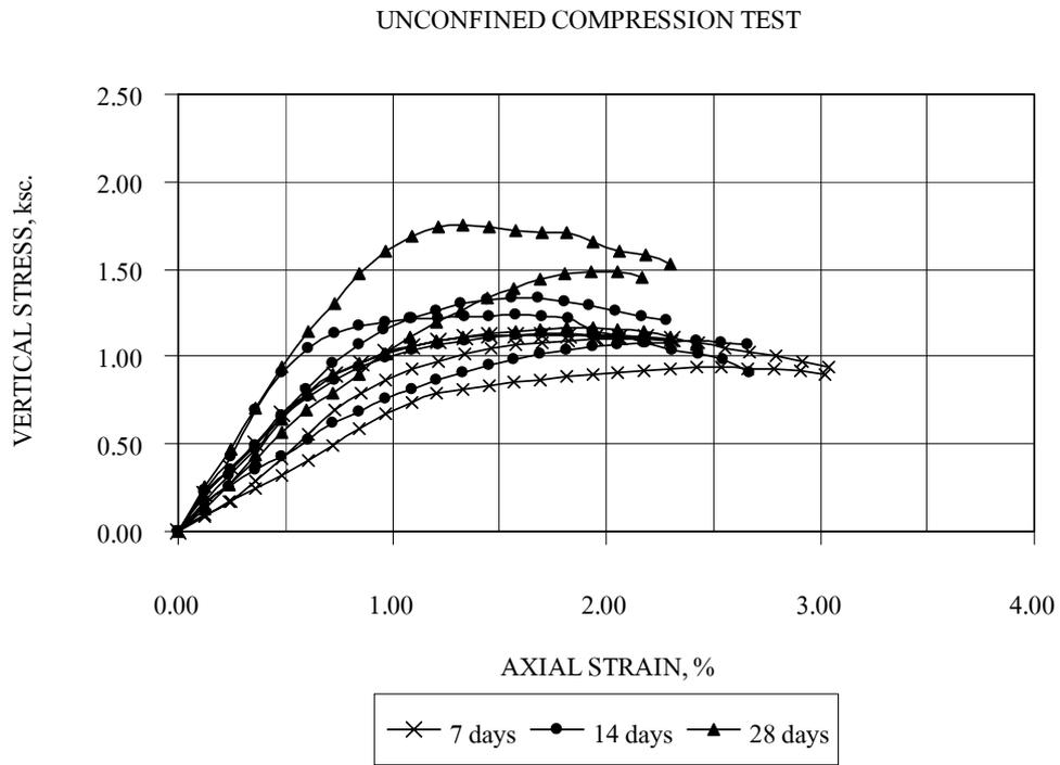
Appendix Figure 1 Stress-strain characteristics of SC108/100
