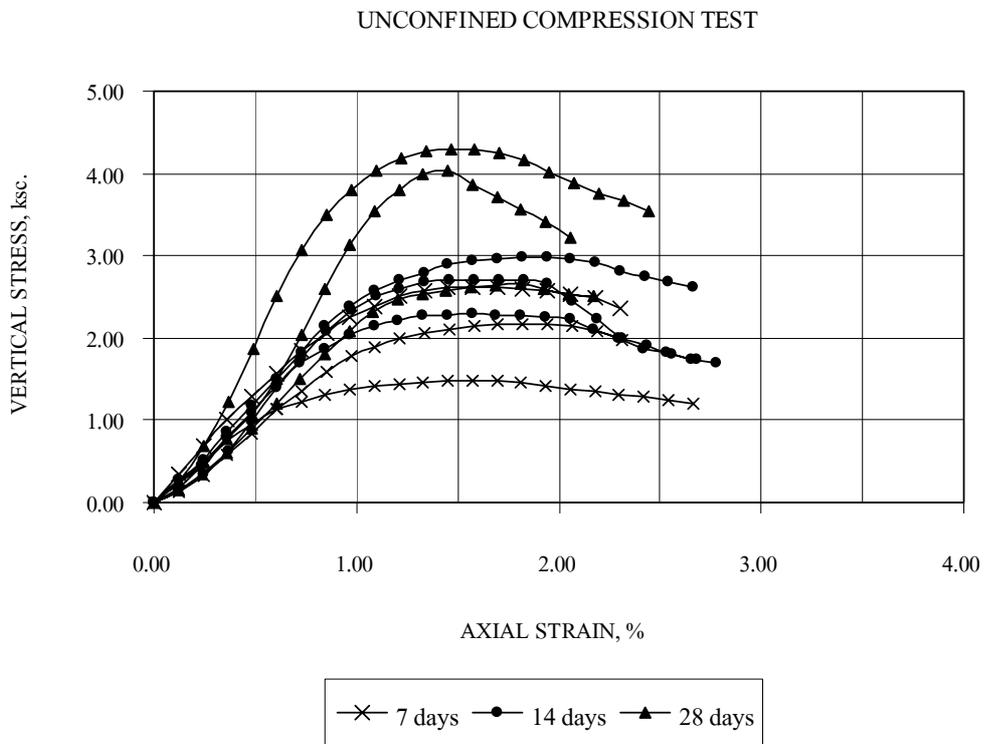
Appendix Figure 2 Stress-strain characteristics of SC108/125
