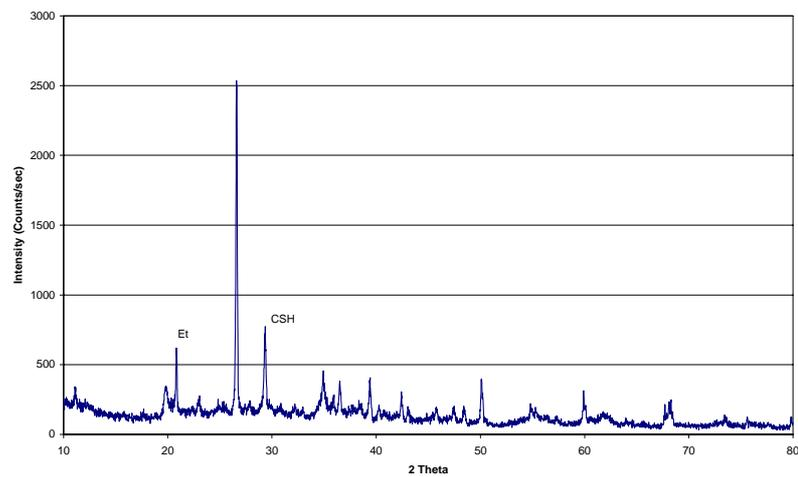
**Figure 55** XRD pattern of cement-stabilized mixture, SC137/150 (7 days)
