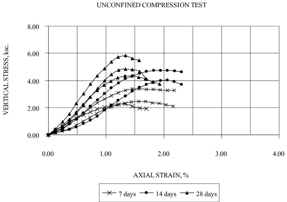
Appendix Figure 3 Stress-strain characteristics of SC108/150
