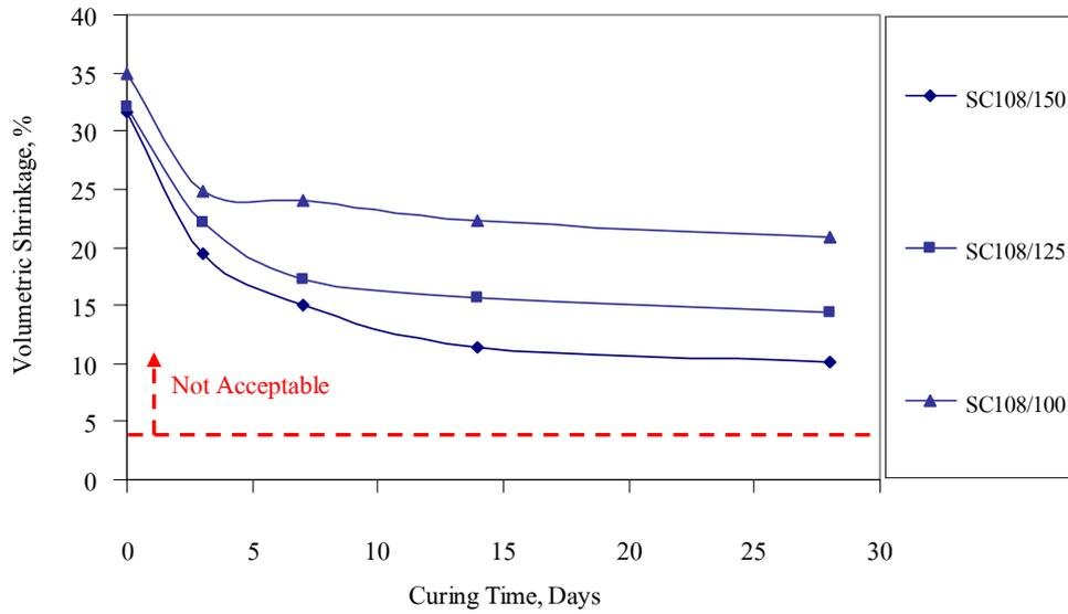
**Figure 31** Volumetric shrinkage of cement mixed dredged materials with curing time (initial water content before mixing was 108.99 %)
