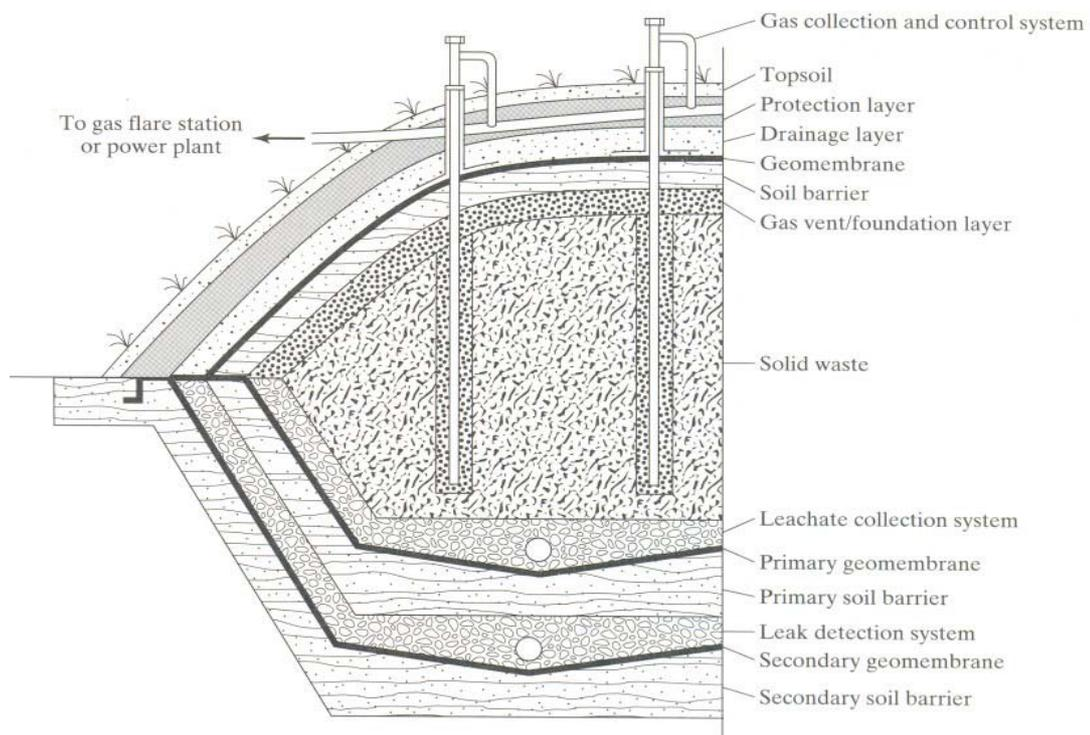
**Figure 6** Schematic Diagram of a Municipal Solid Waste Landfill Containment System
