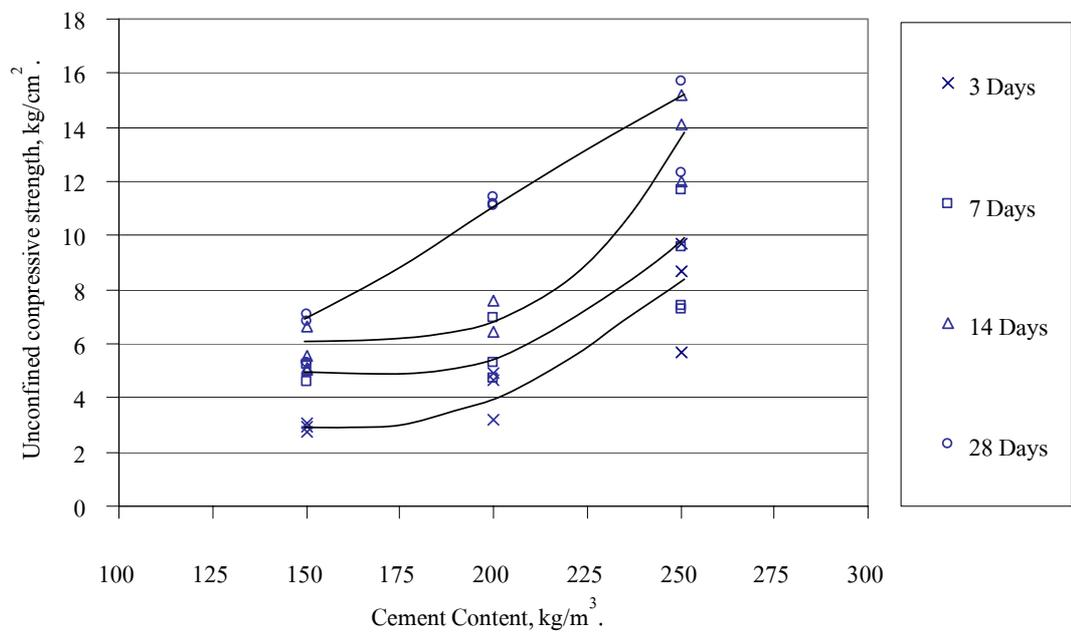
**Figure 24** Unconfined compressive strength of cement mixed dredged materials with cement content (initial water content before mixing was 137.87 %)
