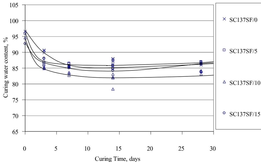
**Figure 41** Curing water content of cement and silica fume mixed dredged materials with curing time (initial water content before mixing was 137.87%)
