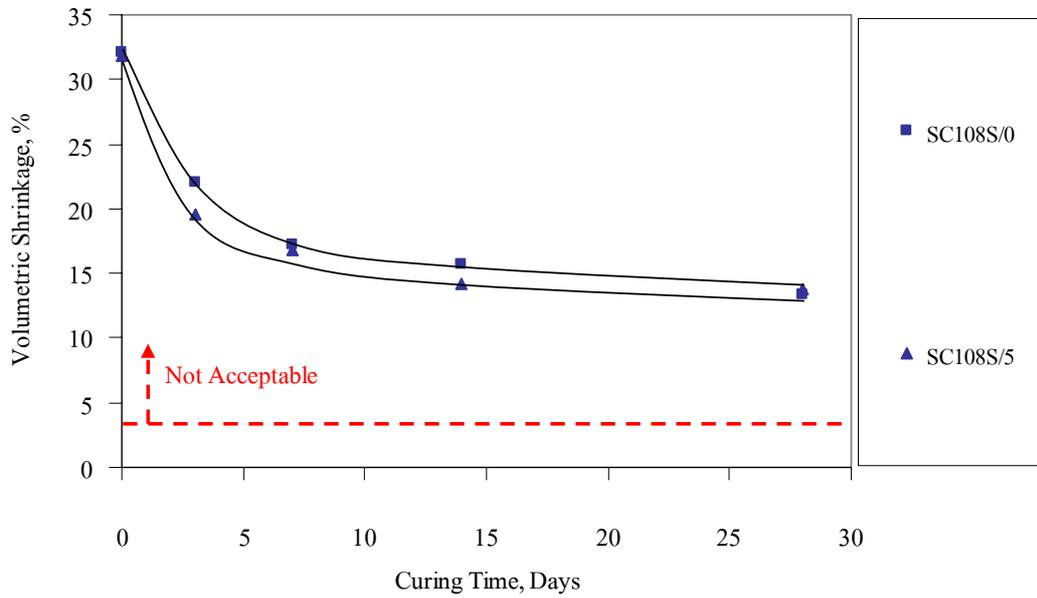
Figure 44 Volumetric shrinkage of cement and sand mixed dredged materials with sand content (initial water content before mixing is 108.99%)
