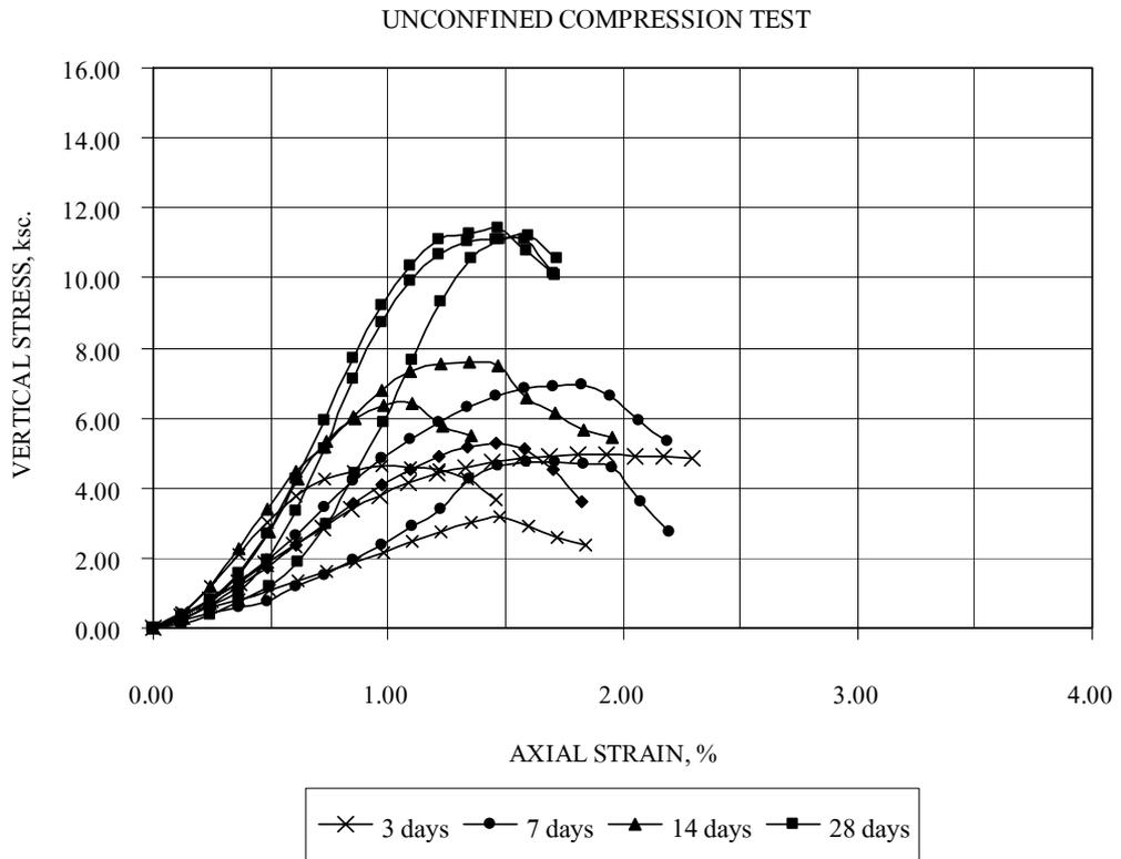
Appendix Figure 5 Stress-strain characteristics of SC137/200
