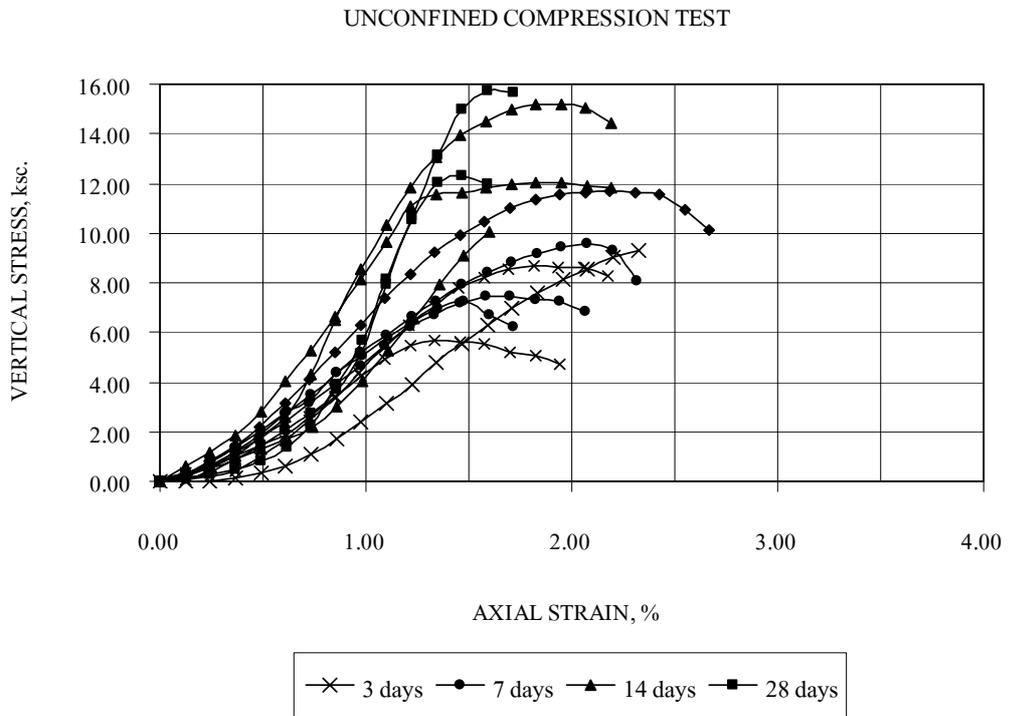
Appendix Figure 6 Stress-strain characteristics of SC137/250
