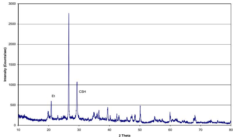
**Figure 64** XRD pattern of cement-stabilized mixture, SC137SF/10 (14 days)
