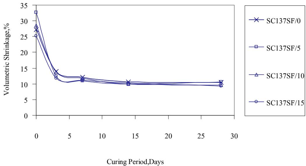
**Figure 39** Volumetric shrinkage of cement and silica fume mixed dredged materials with curing time (initial water content before mixing was 137.87%)
