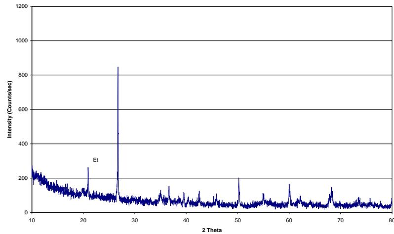
**Figure 52** XRD pattern of cement-stabilized mixture, SC108/125 (14 days)
