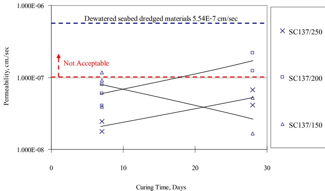
**Figure 27** Permeability of cement mixed dredged materials with curing time (initial water content before mixing was 137.87 %)
