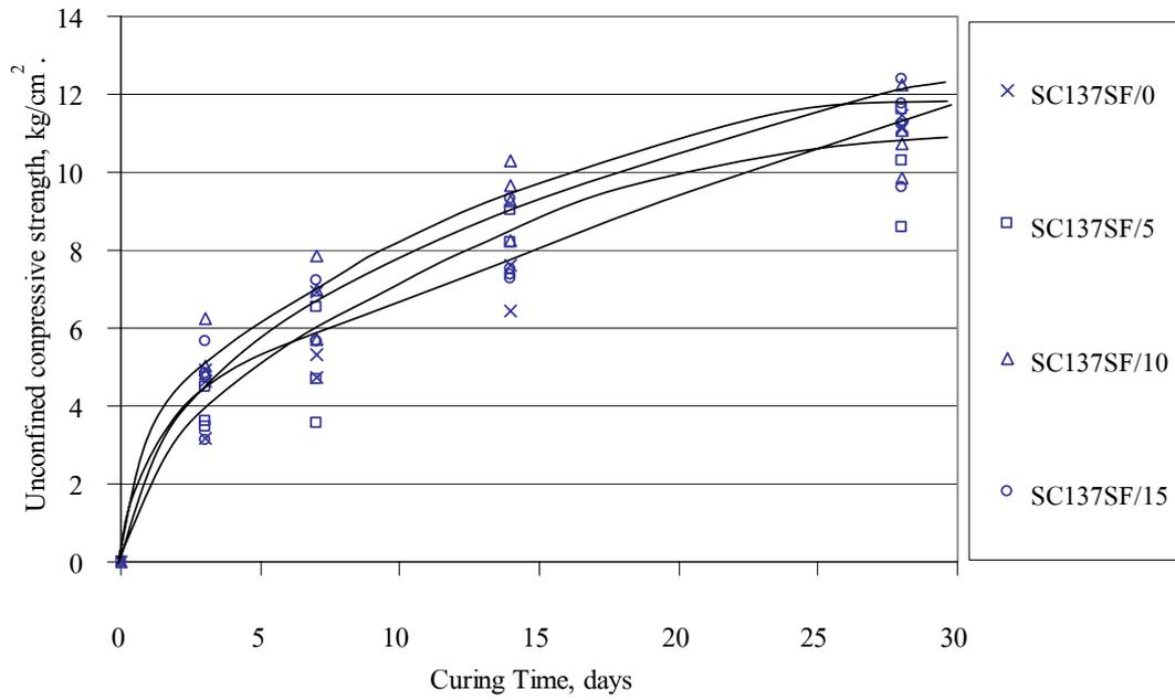
**Figure 35** Unconfined compressive strength of cement and silica fume mixed dredged materials with curing time (initial water content before mixing was 137.87 %)
