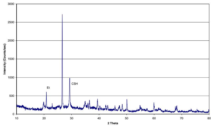
**Figure 65** XRD pattern of cement-stabilized mixture, SC137SF/10 (28 days)
