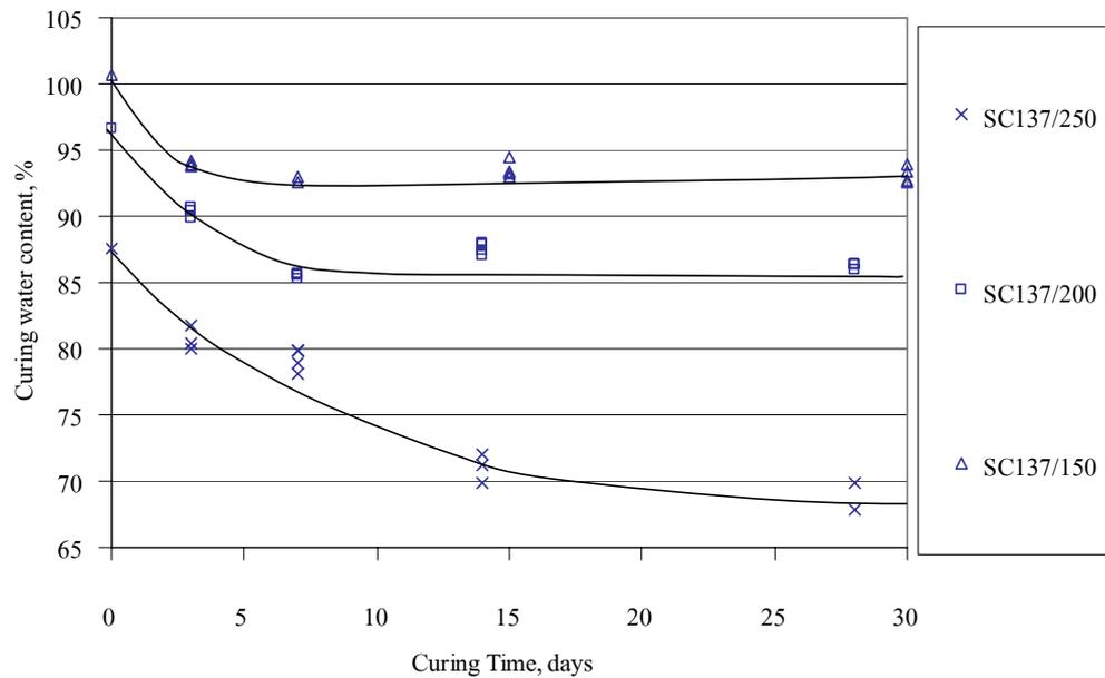
**Figure 34** Curing water content of cement mixed dredged materials with curing time (initial water content before mixing was 137.87%)
