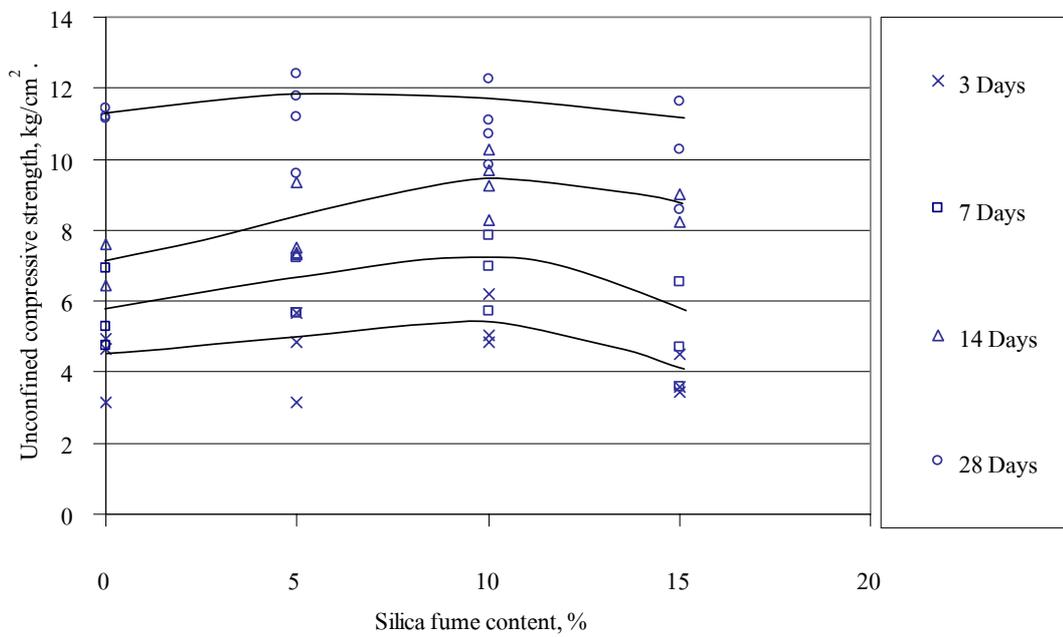
**Figure 36** Unconfined compressive strength of cement and silica fume mixed dredged materials with silica fume content (initial water content before mixing was 137.87 %)
