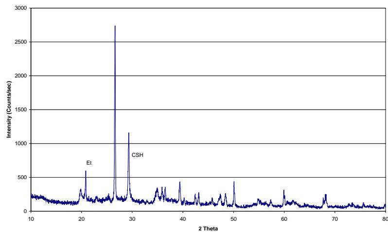
**Figure 56** XRD pattern of cement-stabilized mixture, SC137/150 (15 days)
