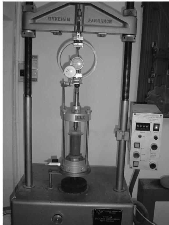
Figure 12 Unconfined compression test apparatus
