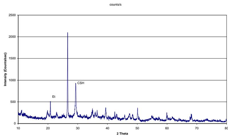
**Figure 60** XRD pattern of cement-stabilized mixture, SC137/250 (14 days)
