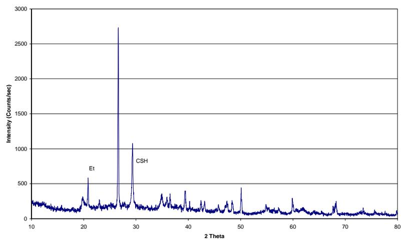
**Figure 63** XRD pattern of cement-stabilized mixture, SC137SF/10 (7 days)
