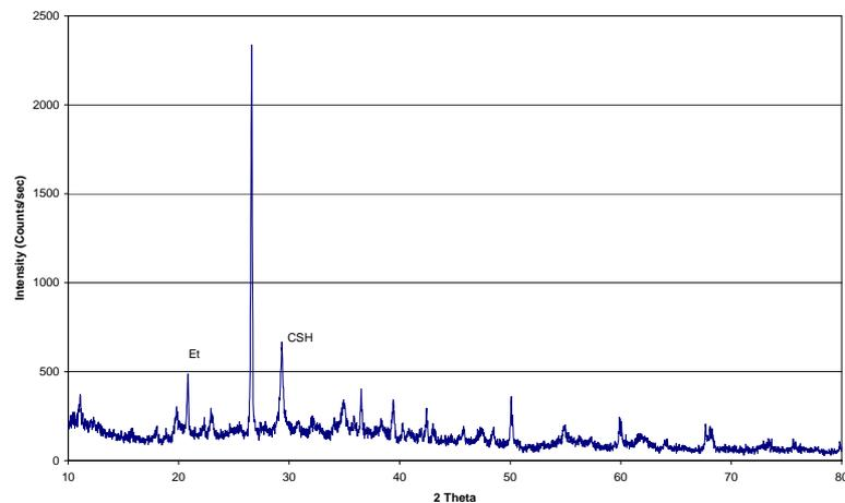
**Figure 58** XRD pattern of cement-stabilized mixture, SC137/250 (3 days)
