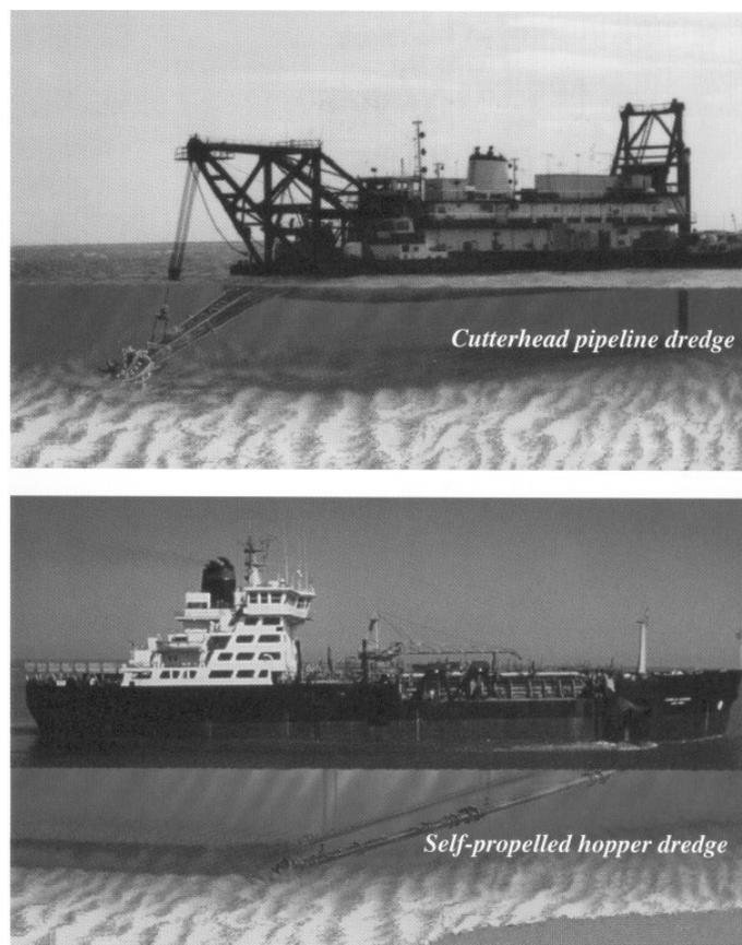
Figure 3 Hydraulic dredges, cutter head pipeline dredge and self-propelled hopper dredge
