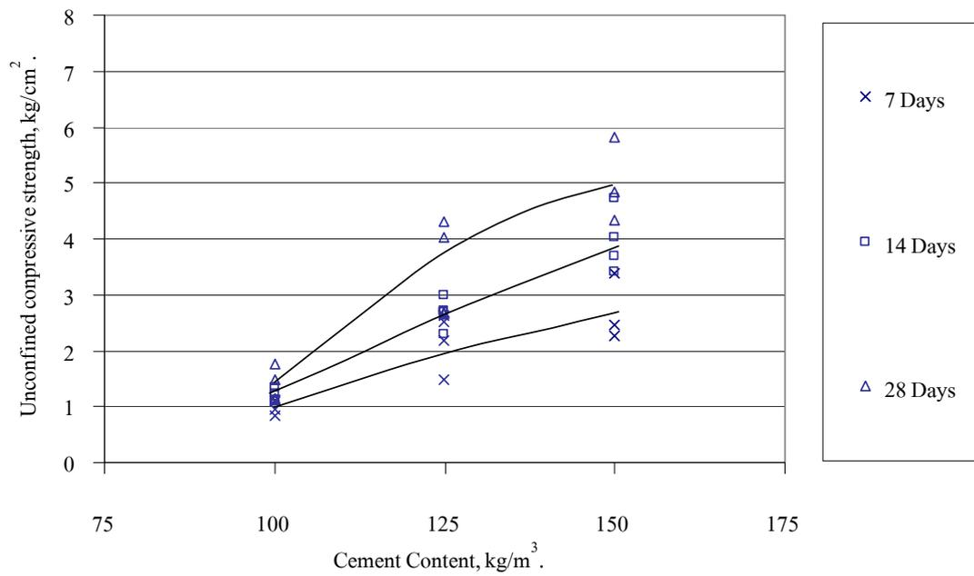
**Figure 23** Unconfined compressive strength of cement mixed dredged materials with cement content (initial water content before mixing was 108.99%)
