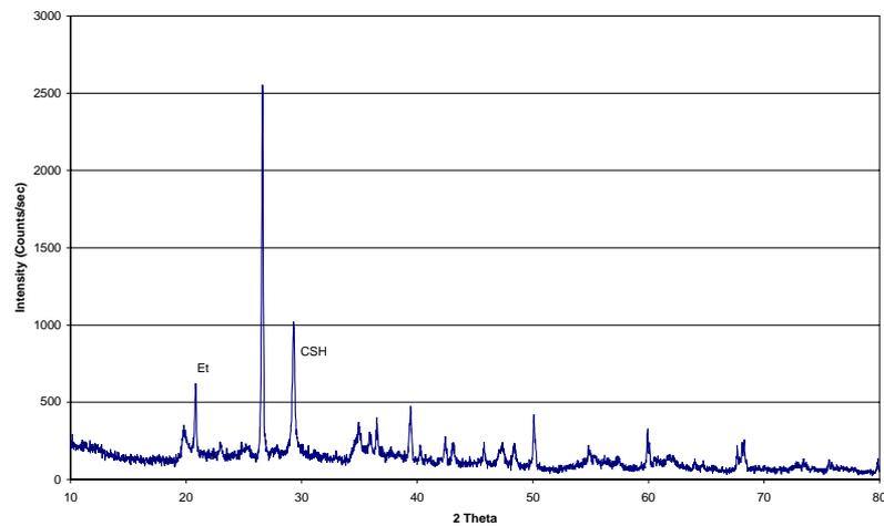
**Figure 57** XRD pattern of cement-stabilized mixture, SC137/150 (30days)
