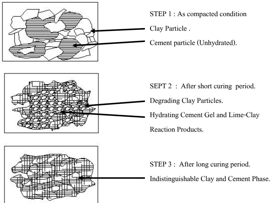
Figure 5 Soil cement structure as suggested by Mitchell and Jack (1966)
