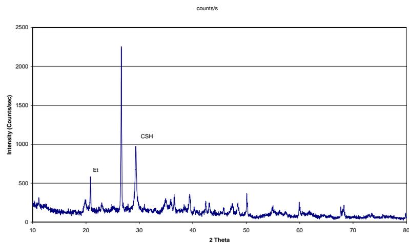
**Figure 61** XRD pattern of cement-stabilized mixture, SC137/250 (28 days)
