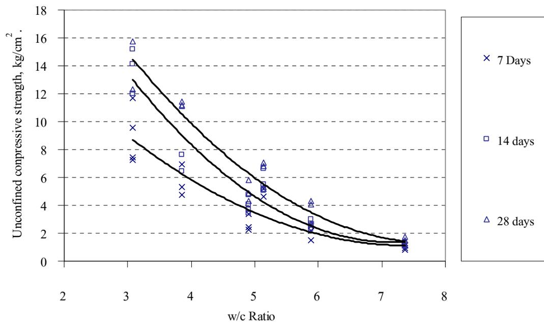
**Figure 25** Unconfined compressive strength of cement mixed dredged materials with w/c ratio.
