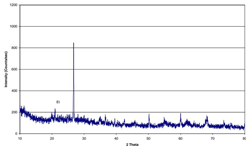
**Figure 53** XRD pattern of cement-stabilized mixture, SC108/125 (28 days)
