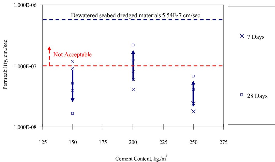
**Figure 29** Permeability of cement mixed dredged materials with cement content (initial water content before mixing was 137.87%)
