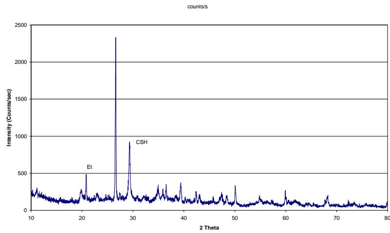
**Figure 59** XRD pattern of cement-stabilized mixture, SC137/250 (7 days)
