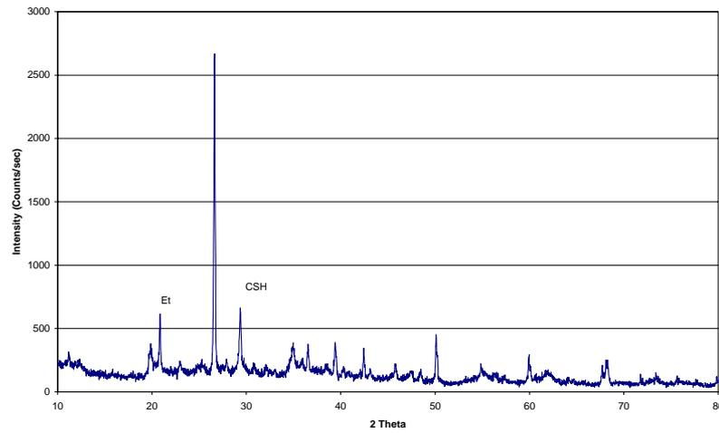
**Figure 54** XRD pattern of cement-stabilized mixture, SC137/150 (3 days)
