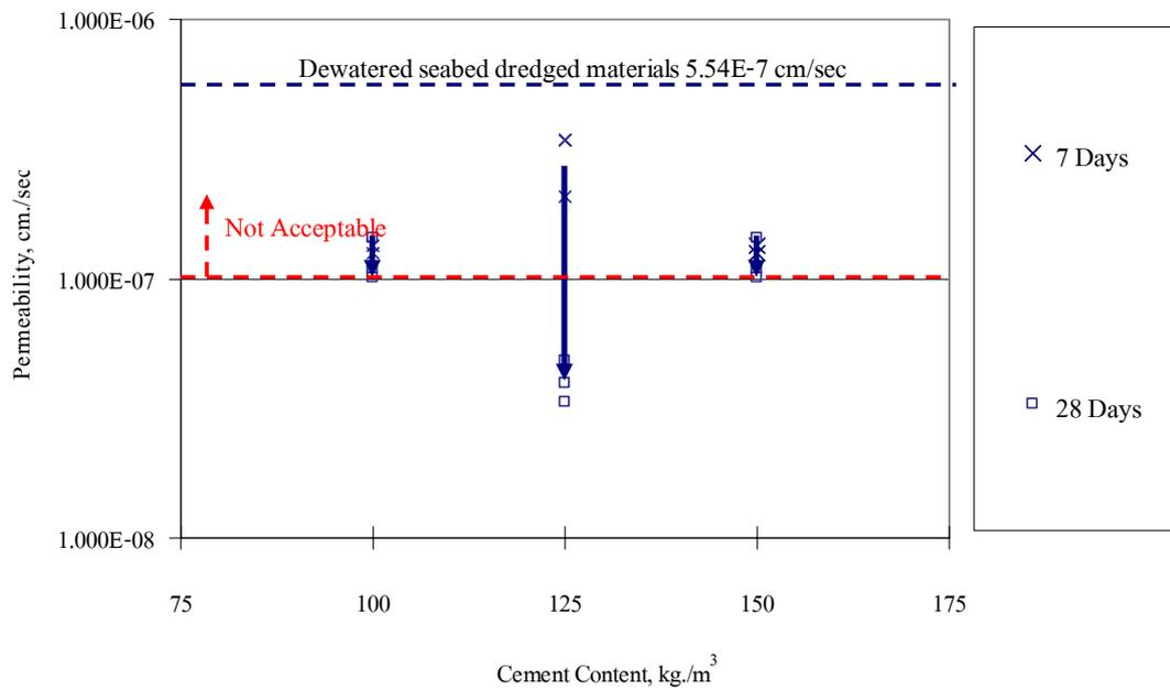
**Figure 28** Permeability of cement mixed dredged materials with cement content (initial water content before mixing was 108.99%)
