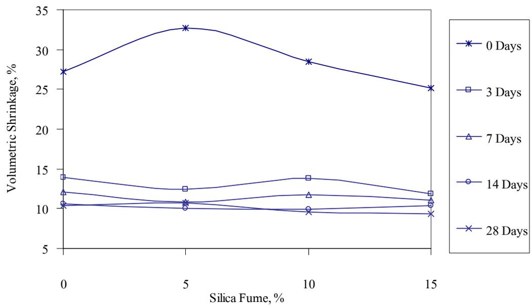
**Figure 40** Volumetric shrinkage of cement and silica fume mixed dredged materials with silica fume content (initial water content before mixing is 137.87%)
