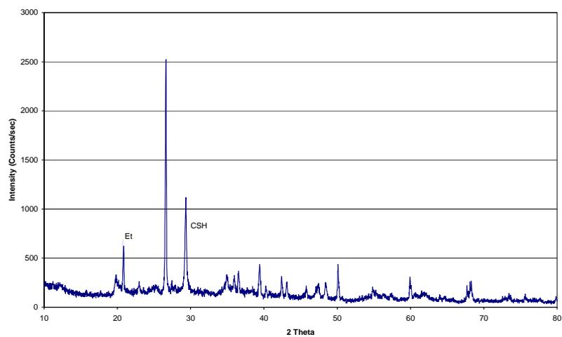
**Figure 62** XRD pattern of cement-stabilized mixture, SC137SF/10 (3 days)
