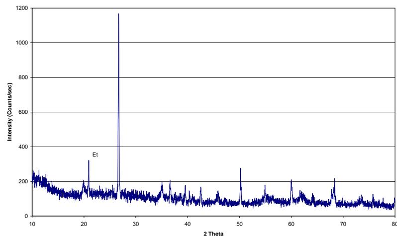
**Figure 51** XRD pattern of cement-stabilized mixture, SC108/125 (7 days)
