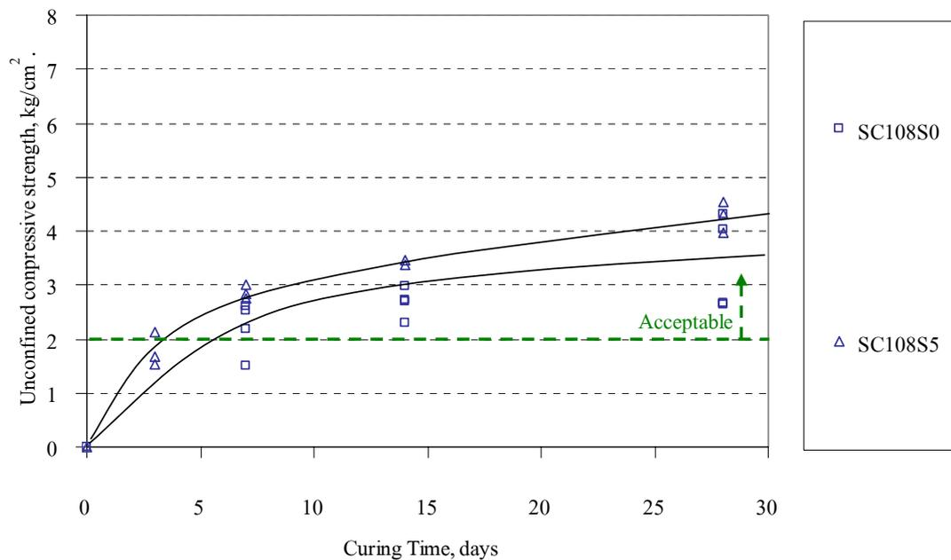
**Figure 42** Unconfined compressive strength of cement and sand mixed dredged materials with curing time (initial water content before mixing is 108.99%)
