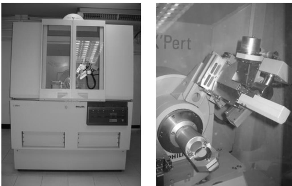
Figure 16 X-ray Diffractometer (Philips X'Pert) for chemical analysis
