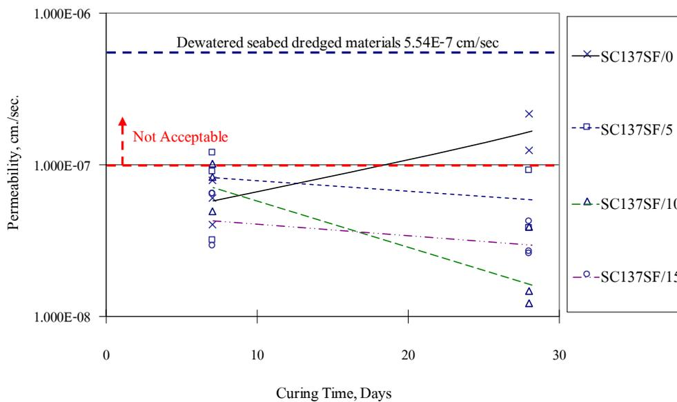
**Figure 37** Permeability of cement and silica fume mixed dredged materials with curing time (initial water content before mixing was 137.87%)
