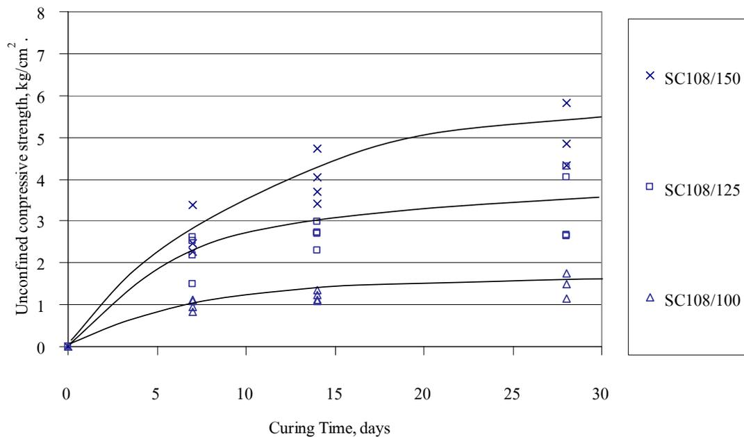
**Figure 21** Unconfined compressive strength of cement mixed dredged materials with curing time (initial water content before mixing was 108.99 %)
