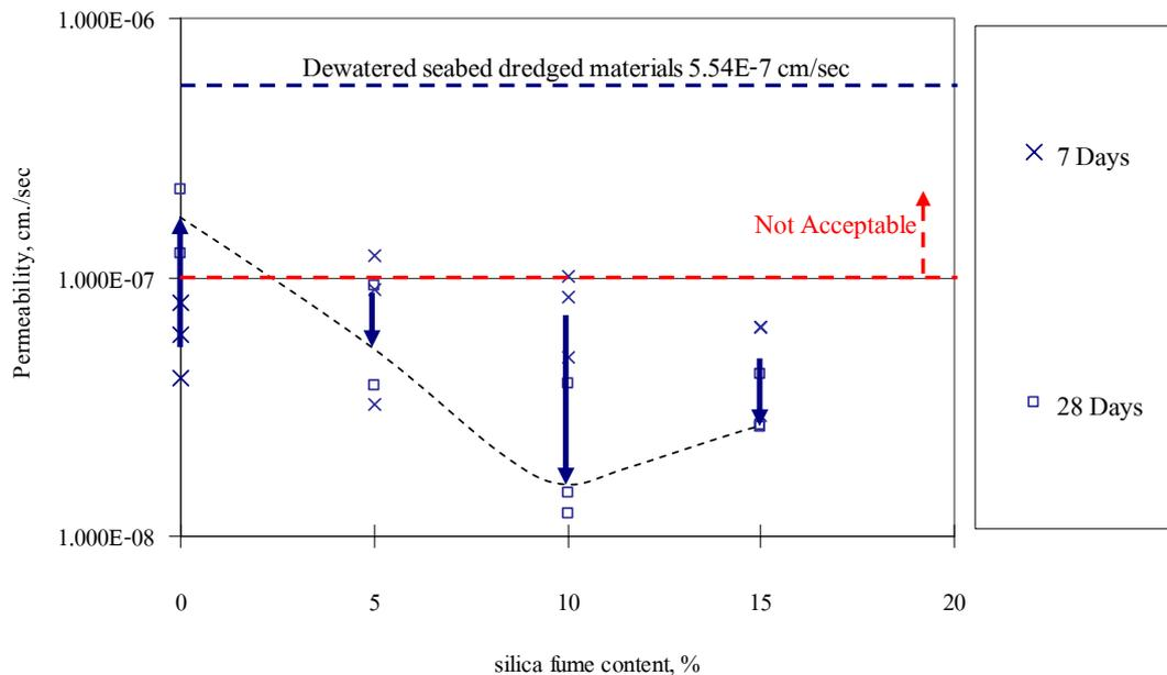
**Figure 38** Permeability of cement and silica fume mixed dredged materials with silica fume content (initial water content before mixing was 137.87%)
