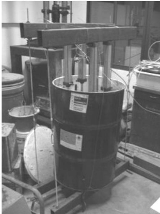
Figure 11 Laboratory dewatering apparatus
