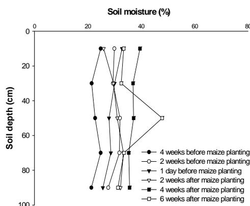
**Appendix Figure 2** Soil field moisture content in Lb soil before and after maize planting (5 May to 3 July, 2005).
