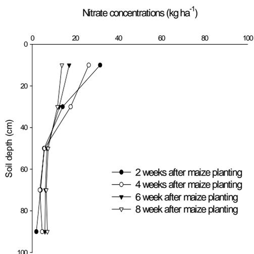
**Figure 20**  $\text{NO}_3^-$ -N distribution in the control treatment of Pc soil series postplant sampling.
