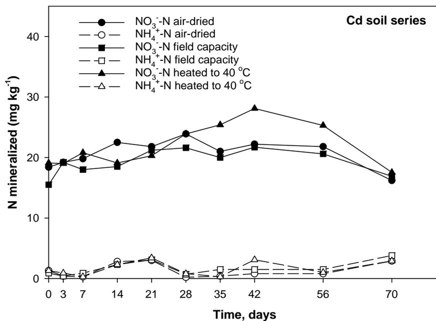
**Figure 5** Nitrogen mineralization ( $\text{NH}_4^+$ -N and  $\text{NO}_3^-$ -N) in the Cd soil as affected by selected pre-treatments under aerobic incubation.
