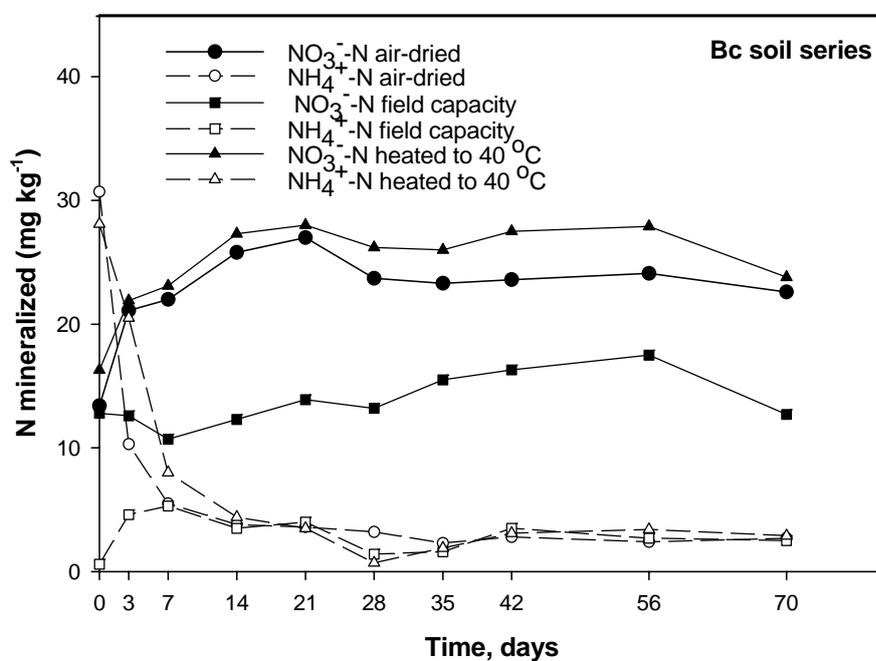
**Figure 11** Nitrogen mineralization ( $\text{NH}_4^+$ -N and  $\text{NO}_3^-$ -N) in the Bc soil as affected by selected pre-treatments under aerobic incubation.
