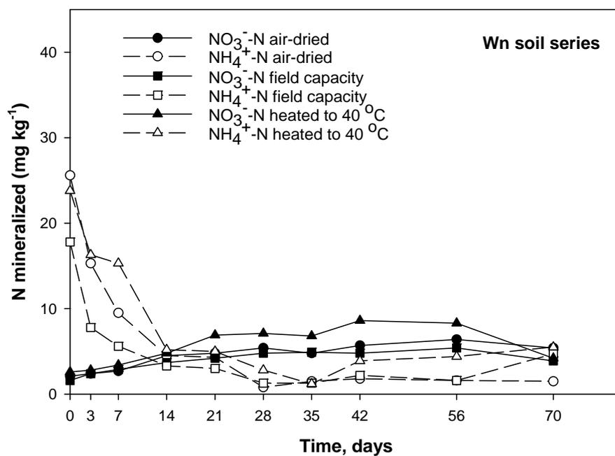
**Figure 10** Nitrogen mineralization ( $\text{NH}_4^+$ -N and  $\text{NO}_3^-$ -N) in the Wn soil as affected by selected pre-treatments under aerobic incubation.
