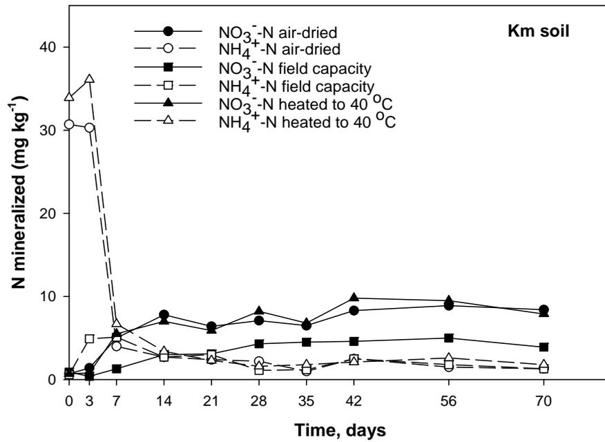
**Figure 12** Nitrogen mineralization (NH<sub>4</sub><sup>+</sup>-N and NO<sub>3</sub><sup>-</sup>-N) in the Km soil as affected by selected pre-treatments under aerobic incubation.
