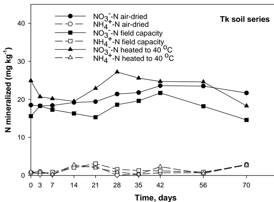
**Figure 6** Nitrogen mineralization ( $\text{NH}_4^+$ -N and  $\text{NO}_3^-$ -N) in the Tk soil as affected by selected pre-treatments under aerobic incubation.
