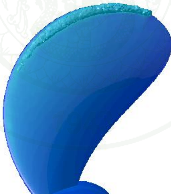
Figure 22 Cavitation on the propeller at cavitation number \sigma = 3 and advance ratio J = 0.5
