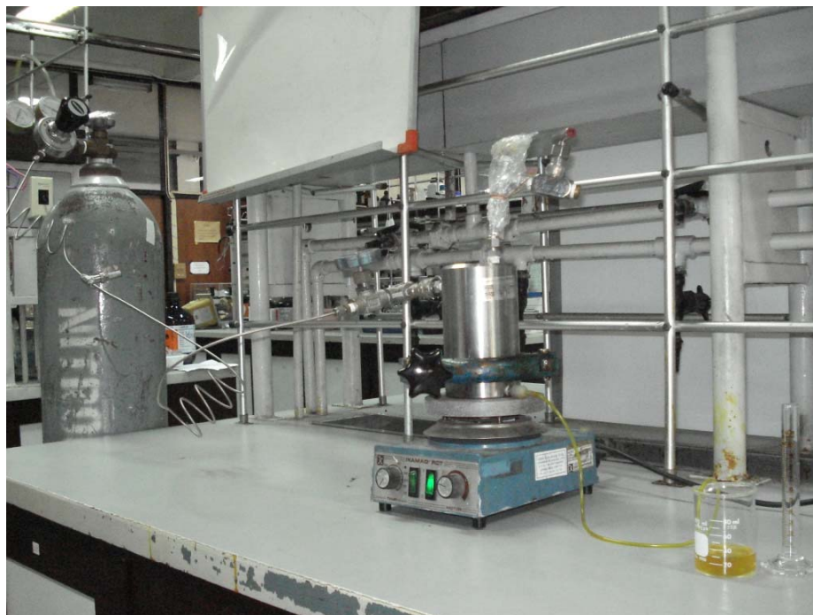
Figure 10 Membrane module set up for recovery sericin from silk cocoon degumming wastewater in this study
