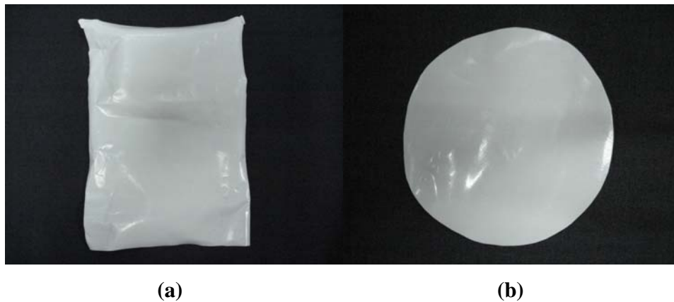
Figure 8 (a) Membrane formation and (b) prepared PSF membrane
