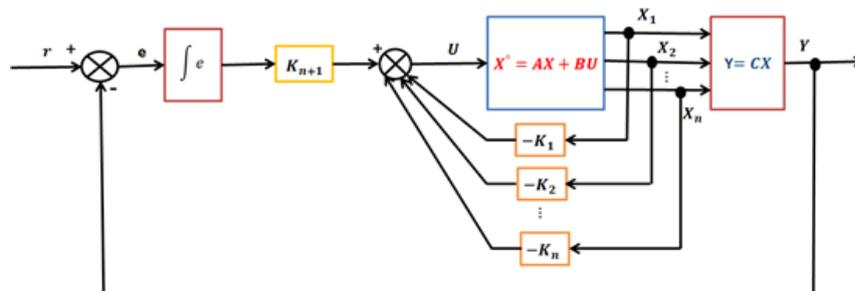
Figure 2. A block diagram of the LQI method
