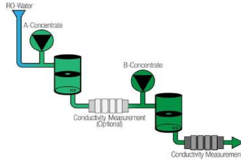
Figure 1. A schematic diagram of dialysate preparation (Måns, 2016)
