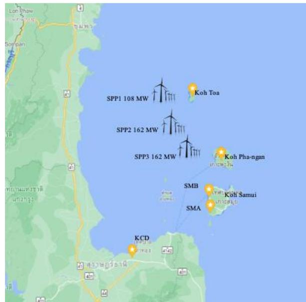
Figure 2. The approximate locations and installation capacities of offshore wind farms and the 115-kV PEA buses: SMA, SMB, and KCD
