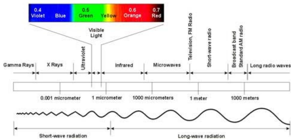
Figure 2 Spectrum of electromagnetic energy.
